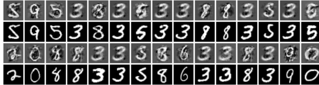
Figure 3: Top 30 reconstructed samples from MNIST dataset. Odd rows show reconstructed samples and even rows show the corresponding training sample. The neural network was trained on 500 MNIST images. It is obvious from the figure that the background pixels did not reconstruct well.
