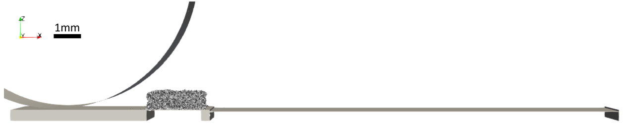
Figure 1: Simulation setup with roller, fully extended powder reservoir piston with 42,000 particles and powder reservoir
