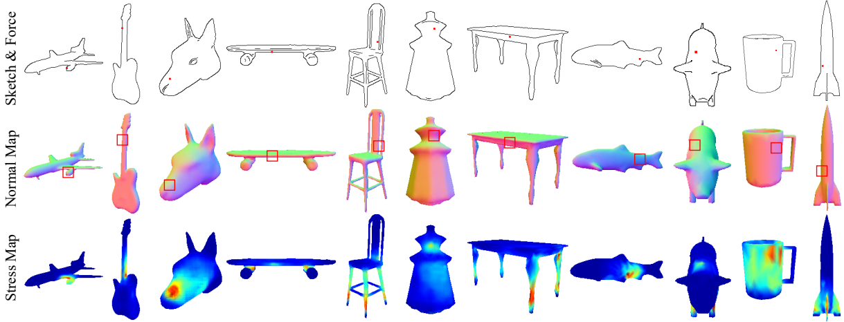
Fig. 9. Result gallery of eleven categories in our synthetic sketch-force-stress data. The top row shows the input sketches and external force locations (plotted as red dots), while the middle and bottom rows are our generated normal maps (with predicted force directions at the center of red boxes) and synthesized stress maps, respectively. Please zoom in to examine the details of the applied force locations/directions and the generated structural stress results.
