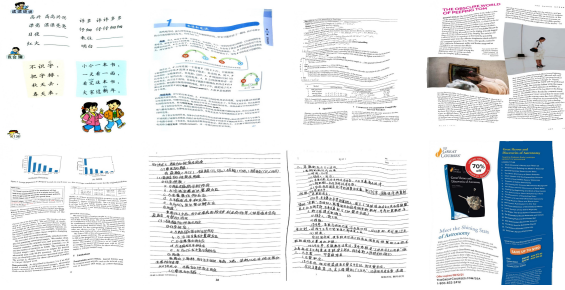
Figure 12. Geometrically-distorted document images resulting from our randomly-generated flow fields.
