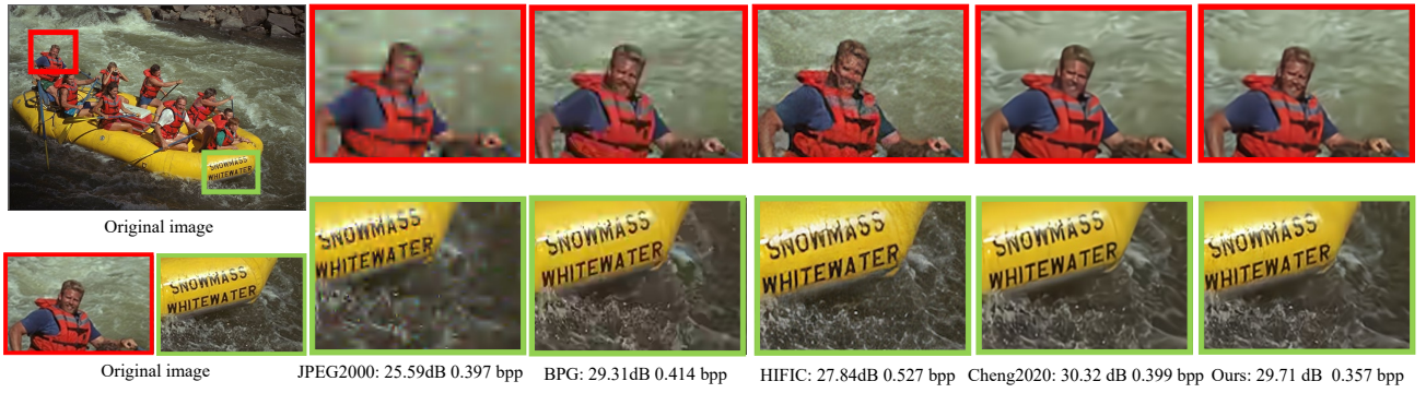
Fig. 9. Visual comparison of reconstructed images from the Kodak dataset. The loss functions of Cheng2020 and ours are MSE losses.
