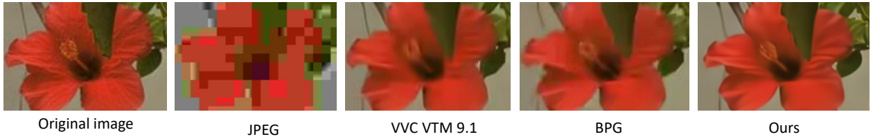
Fig. 10. Visual comparison between the traditional methods and ours from the Kodak dataset.
