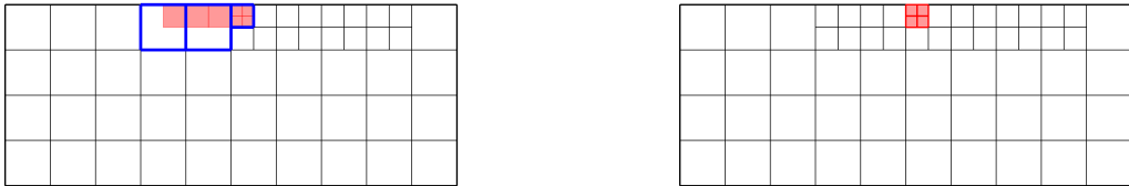
(a) The Q \in \mathcal{Q}^+ highlighted on top of \mathcal{Q}_n^+ (red) and the overlapping elements from \mathcal{Q}_n (blue). (b) Illustration of over-refinement in \mathcal{Q}_{n+1} . The highlighted elements do not impact the basis cardinality for polynomial degrees p \geq 2 .
