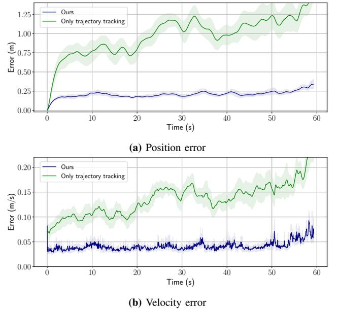
**Fig. 5:** Our method’s performance compared to only the trajectory-tracking control. The curves show the mean error across 20 episodes with corresponding 95% confidence interval.
