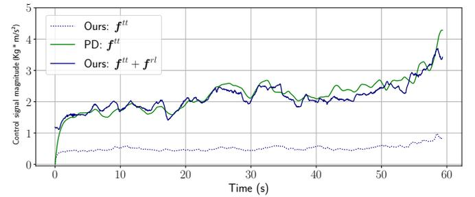
**Fig. 6:** Magnitude of the control signal. Solid lines show the total action signal for our method (blue) and only the trajectory-tracking control (green). Additionally, we show the isolated tracking-trajectory component of our method (dotted blue).
