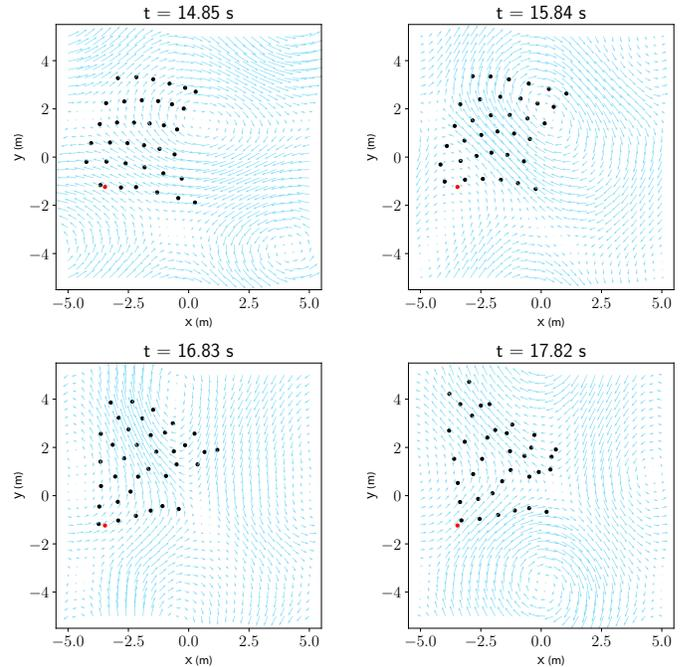
**Fig. 1:** A team of 36 robots navigating in turbulent wind. The robots are trying to maintain a square formation using only a trajectory-tracking controller. Blue arrows show the wind vector field. The red dot shows the target location of the bottom-left robot in the formation. The X-axis and y-axis units are in meters.
