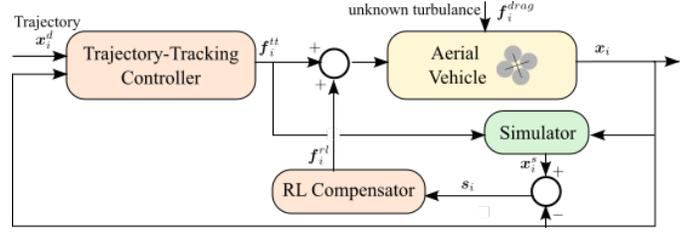
Fig. 2: Control diagram of our proposed method.
