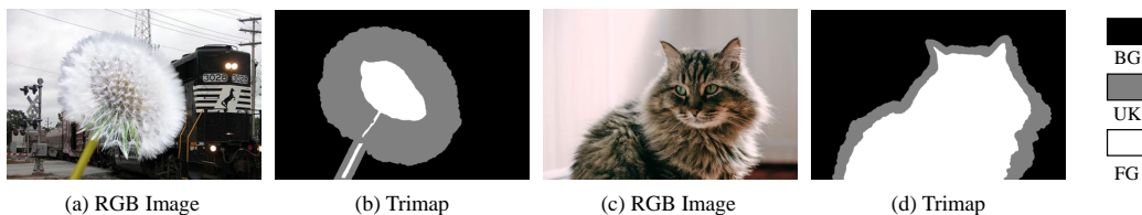
Figure 2: RGB Image and Trimap. The trimap divides an image into foreground (FG), background (BG), and an unknown region (UK). Algorithms based on the trimap only need to predict the unknown region. This reduces the algorithmic complexity but increases the interactive cost.
