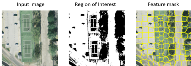
Fig. 2: An example binary threshold mask and feature mask using superpixels [16] generated from an image from UCMerced. Localization XAI metrics need a binary mask for the region of interest and a feature mask is needed for LIME to improve computation.
