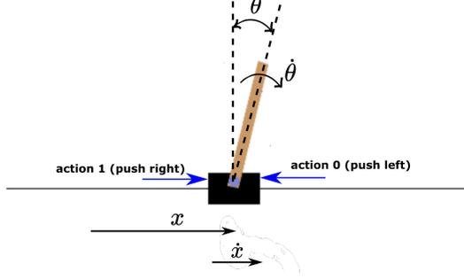
Figure 9: Schematic of the CartPole environment. The state space is parametrized as  $(x, \dot{x}, \theta, \dot{\theta})$ , where  $x$  is the cart position and  $\theta$  is the pole angle. We use the default termination condition as the unsafe set  $\mathcal{X}_{\text{unsafe}} = \{|x| \geq 2.4 \text{ or } |\theta| \geq 12^\circ\}$ .
