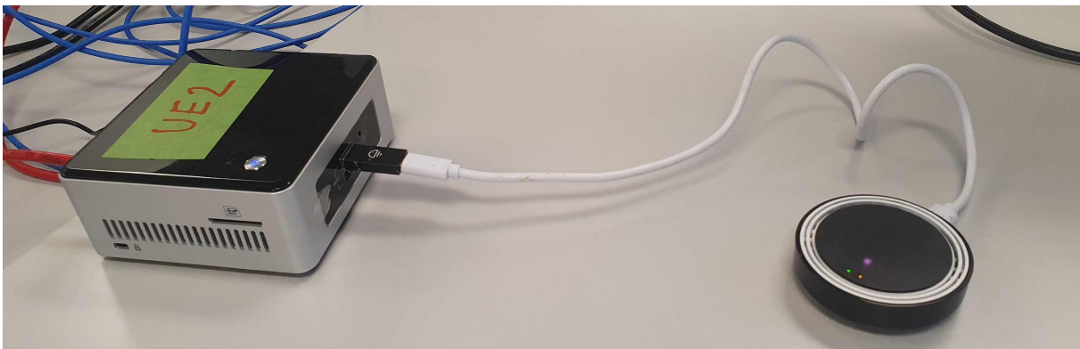
Figure 6: NUC with LiFi receptor dongle.
