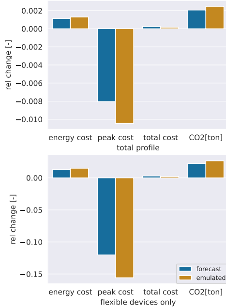
Figure 17: Deviations of different objectives from the simulated results, using the energy oracle to optimize and forecast the power profiles (blue) or to completely bypass the simulation (orange). Top: relative error of objectives normalized with the total simulated costs. Bottom: relative error of objectives normalized with the additional costs faced by the DSO due to the flexible group.
