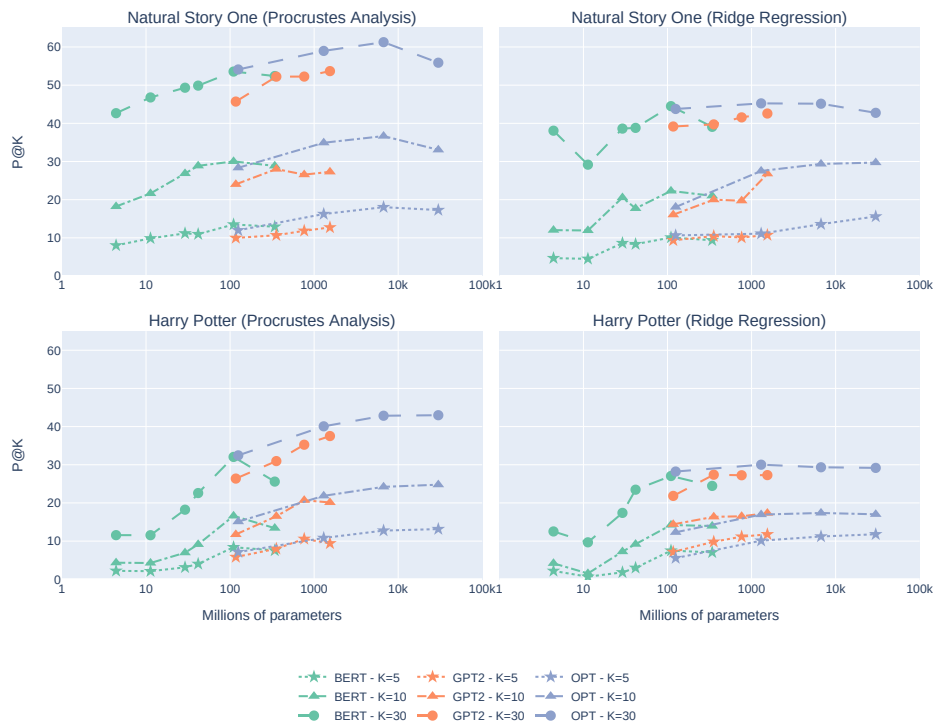
Figure 2: Convergence Results for Three Families of Language Models on Two Datasets. The task for Harry Potter dataset here is: Given a neural response, which word in a vocabulary of 1,291 words, was read at the time the response was recorded? Random retrieval baseline P@10 is less than 1%, while the FastText baseline P@10 is less than 7%. See more details of baselines in Table 2.
