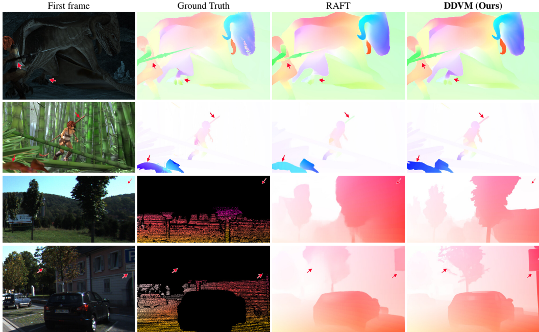
Figure 4: Visual results comparing RAFT with our method after pretraining. Note that our method does much better on fine details and ambiguous regions.
