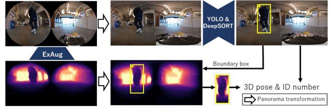
Fig. 3: **Pedestrian detection and tracking.** We use a combination of YOLO and DeepSORT to detect and track pedestrians from visual observations, and estimate their relative position using the scaled depth estimates from ExAug’s perception module.
