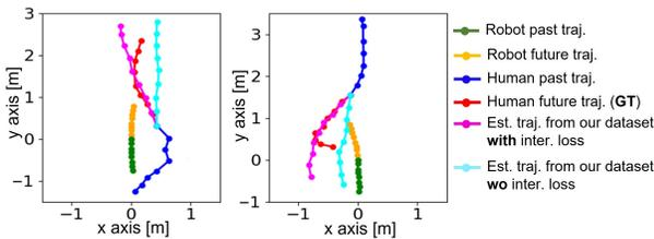
Fig. 9: **Examples of using the learned human dynamics model to predict future human positions,** conditioned on past human positions (blue), past robot positions (green), and future robot plans (yellow). Training with the interaction-enriched dataset (magenta) leads to better predictions than the naïve dataset (cyan).
