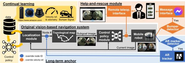
Fig. 4: **HuRoN System overview.** We design our autonomous data collection platform around a vision-based navigation system (gray) that uses a topological graph and a learned control policy. Our proposed system has three key components: a help-and-rescue module for collision recovery (orange), long-term anchors for localization (blue), and continual learning (yellow).
