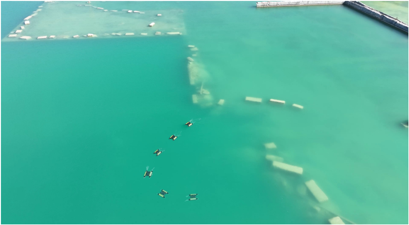
(a) An Autonomous Surface Vehicle is performing elevation information gathering task using a sonar.
