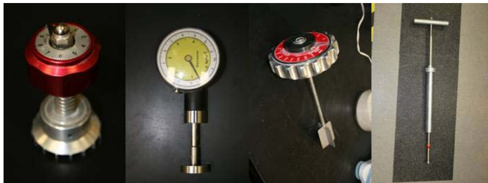
Figure 1. (Left to Right) Pocket vane shear tester, Pocket penetrometer, "Geovane" shear strength tester, and hand-held penetrometer
