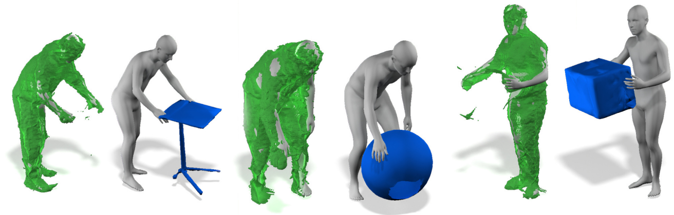
Figure A.4. BEHAVE-Raw. Results of our method on raw point clouds from the BEHAVE dataset. The input point cloud is visualized over the human mesh for reference. The prediction is made using just a point cloud and an object class label.
