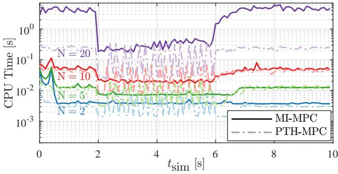
Fig. 4. Computation (CPU) time for the trajectory in Fig. 3a). The solid and dashed lines indicate the MI-MPC and the PTH-MPC controllers, respectively. The  $N$  labels identify the two lines directly above them. Simulations were performed on an Intel(R) Core™ i5 processor running at 2.40 GHz with 15.7 GB of useable RAM.
