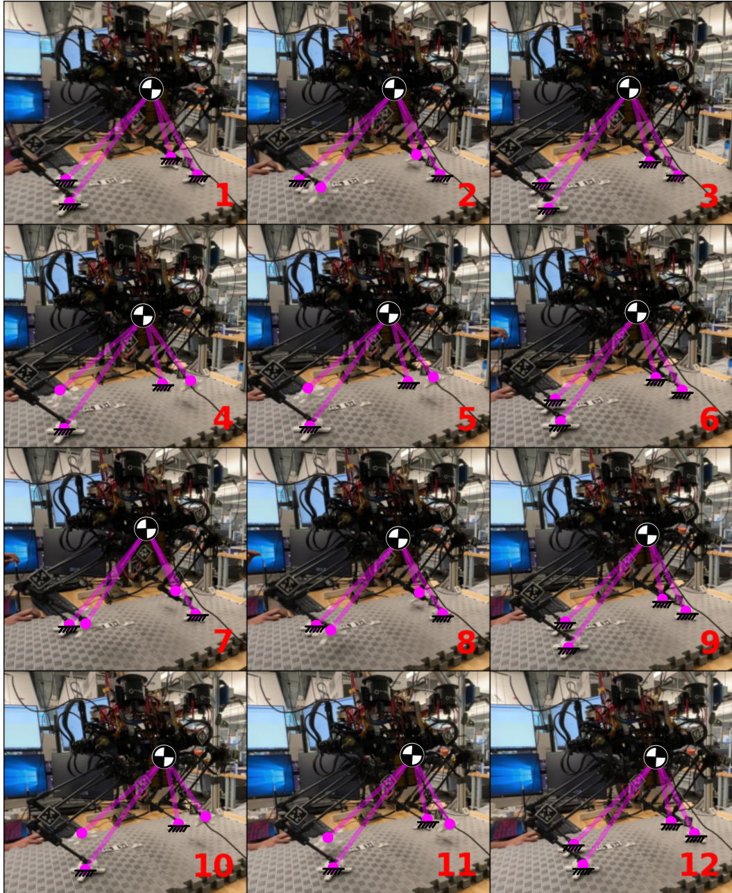
Figure 7.3: The figure provided shows a discrete-time sequence from an experiment involving thruster-assisted trotting in place. The graph displays the observed patterns of legged locomotion during the trial, and the accompanying data specifies the thrust output from the thrusters used in the test.
