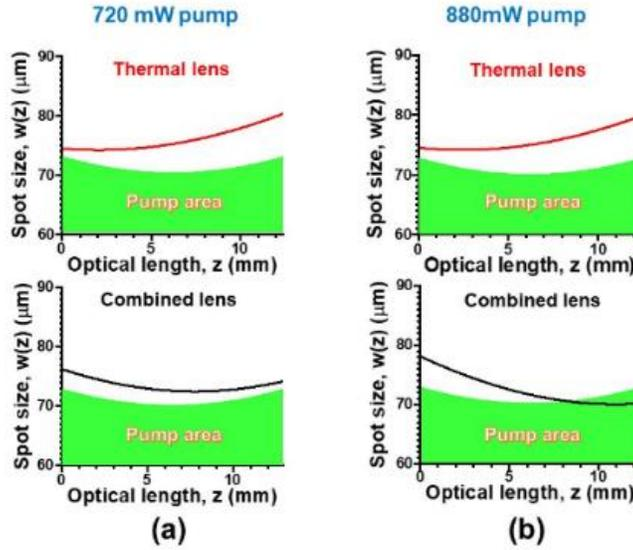
Fig. 6. Spot size variation along the ruby laser crystal with thermal lens (upper traces) and combined lens (lower traces)
