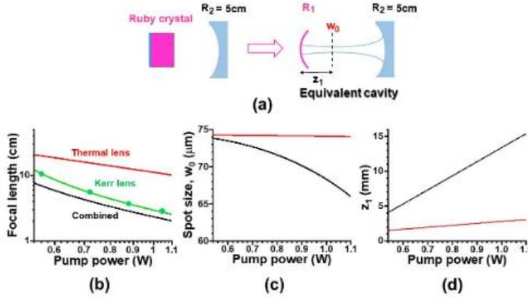
Fig. 5. (a) Equivalent laser-cavity configuration featuring thermal and Kerr lens effects. (b) Pump-dependent focal lengths of thermal, Kerr, and combined lenses. Pump and effective lasing beam spot sizes are assumed to be 72  $\mu\text{m}$ . (c), (d) Pump-dependent beam waist spot size and its position within the cavity.
