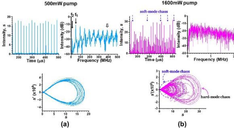
Fig. 3. (a) Quasi-periodic spiking oscillation featuring two competing frequencies,  $f_1 = 9.5$  kHz and  $f_2 = 48.75$  kHz, whose higher harmonic components merge in the vicinity of 390 kHz. (b) Chaotic state featuring alternating soft and hard-mode chaos over time which will be discussed again in section 5.
