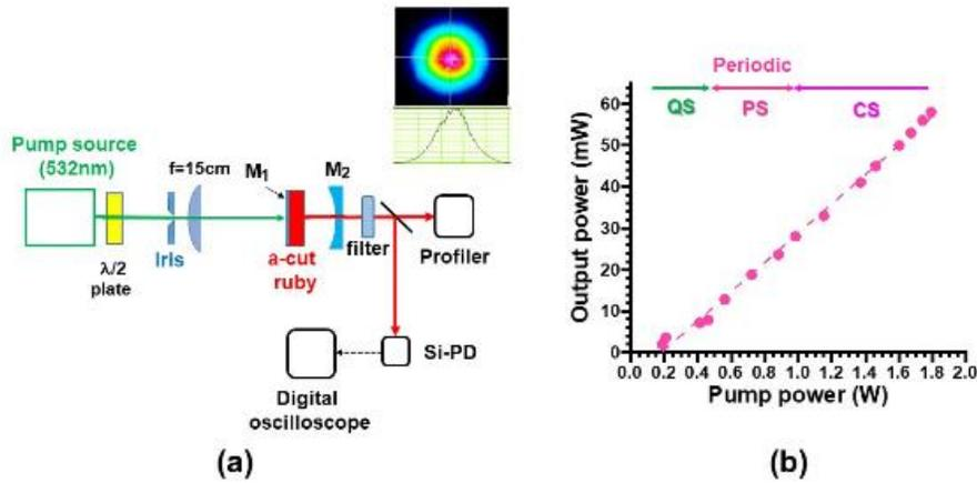
Fig. 1. (a) Experimental apparatus. (b) Input-output characteristics. QS: quasi-periodic spiking regime, PS: periodic spiking regime, CS: chaotic state.
