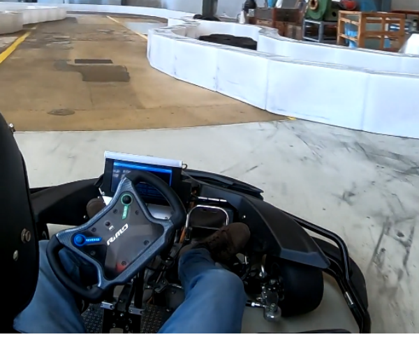
Fig. 12. The real go-kart platform driving autonomously.
