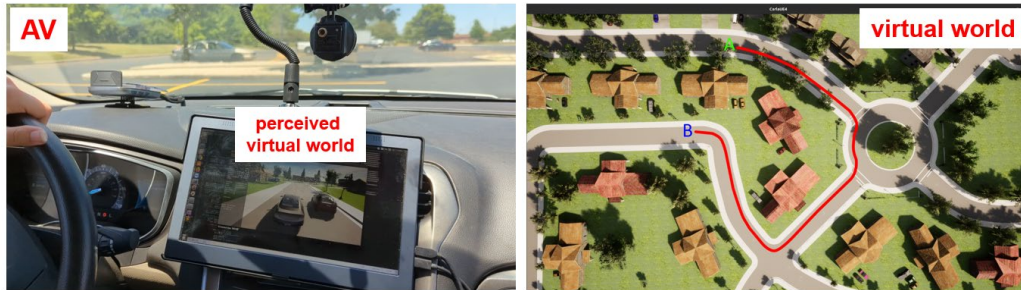
Figure 6. Actual AV in parking lot and planned path in the virtual world.
