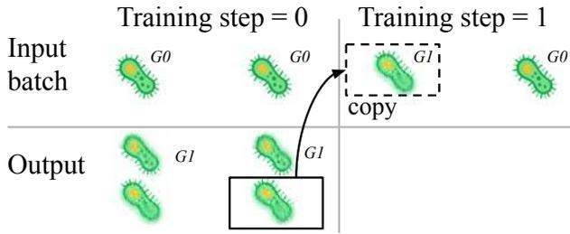
Figure 2: **Batch substitution.** We replace half of the input batch at training step 1 with the output of the NCA at training step 0. This allows the NCA to learn to self-replicate its own output while simultaneously staying close to the target image. There are 8 batches but for simplicity only 2 are shown here.
