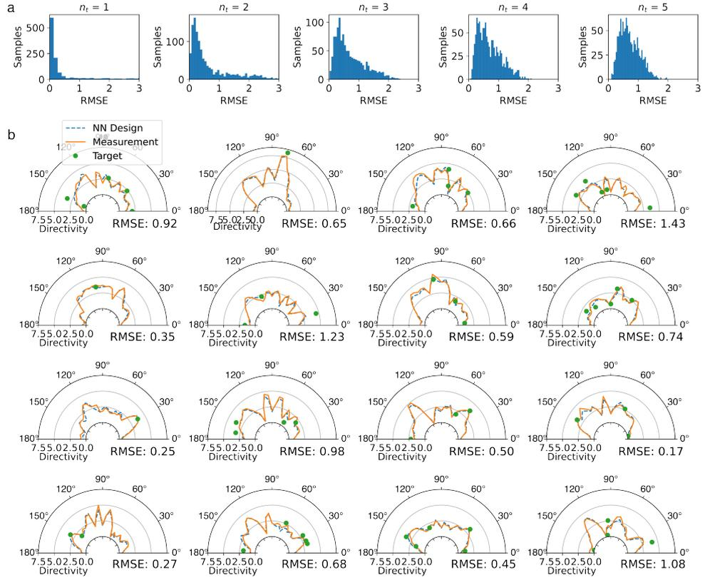
**Extended Data Fig. 4** Performance of the designer for case B. (a) RMSE distribution on sequence with different target number  $n_t$ . (b) Random-selected visual examples, sampling from 6,000 test samples with random seed = 2.
