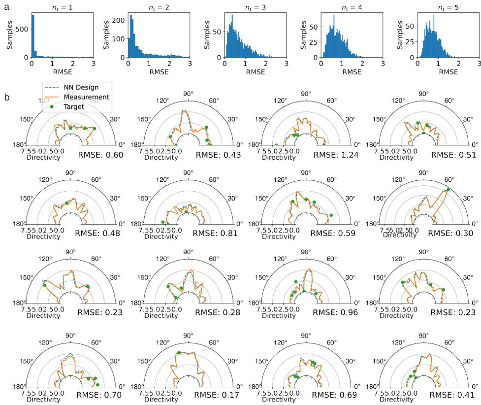
**Extended Data Fig. 3** Performance of the designer for case A. (a) RMSE distribution on sequence with different target number  $n_t$ . (b) Random-selected visual examples, sampling from 6,000 test samples with random seed = 1.
