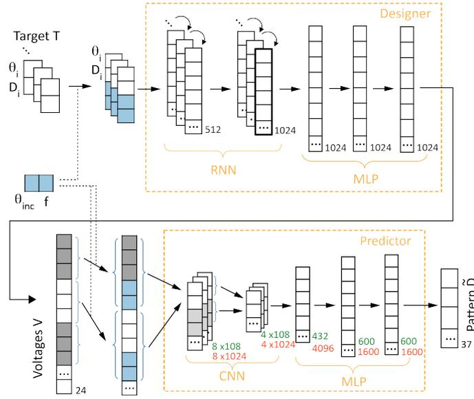
**Extended Data Fig. 1** Proposed sequential tandem network architecture. Dimensions of tensors in the predictor for case A,B and case C,D are in green and red, respectively.
