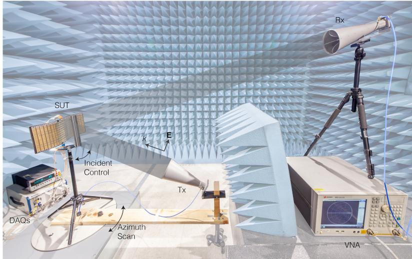
**Fig. 3** Experiment setup for pattern data gathering. The transmission between Tx and Rx through specular reflection on the SUT is recorded by the VNA. By rotating the azimuth scanning motor, Rx equivalently sweep across the azimuth plane to collect the pattern. Incident angle is controlled by a small servo motor the SUT directly mounted on. Three DAQ cards provide the bias voltages for all channels.
