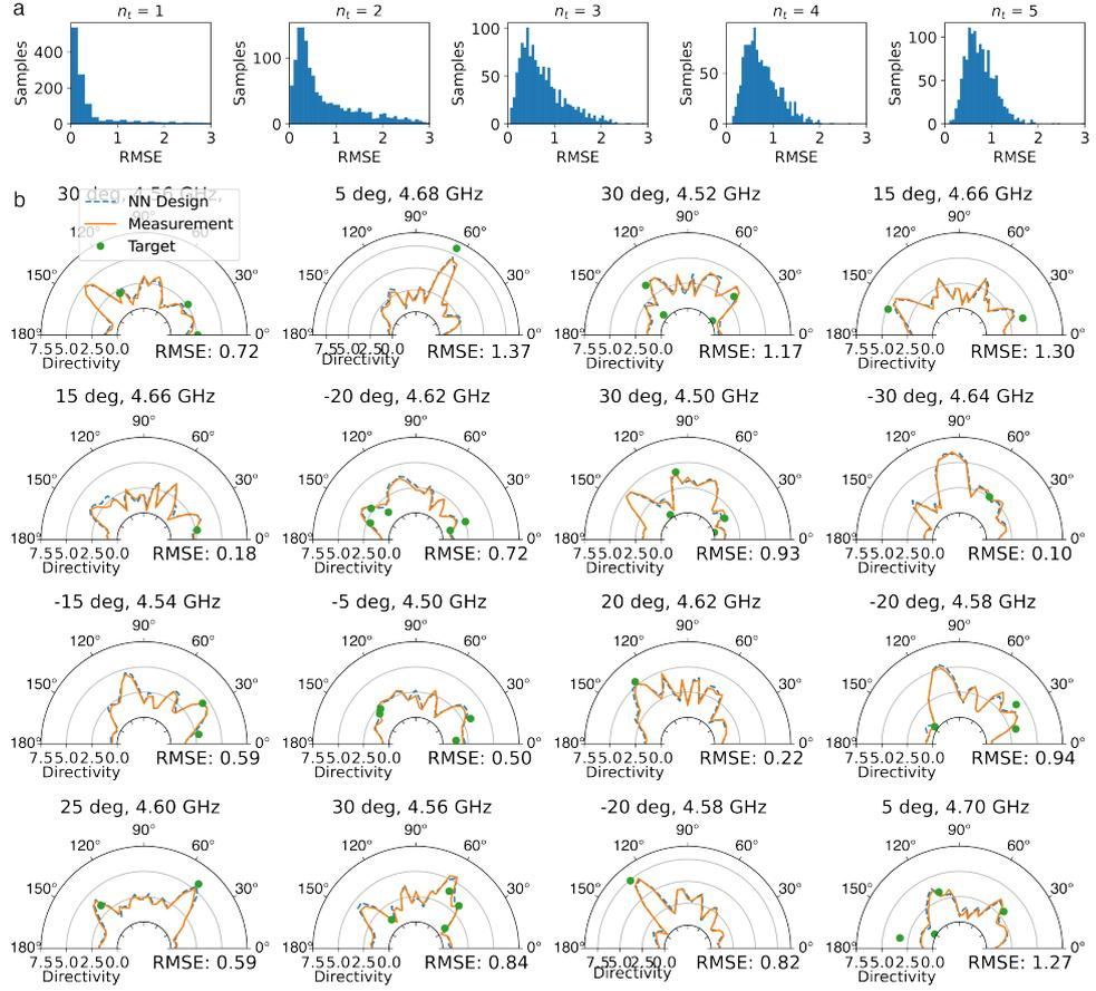
**Extended Data Fig. 6** Performance of the designer for case D. (a) RMSE distribution on sequence with different target number  $n_t$ . (b) Random-selected visual examples, sampling from 6,000 test samples with random seed = 4.
