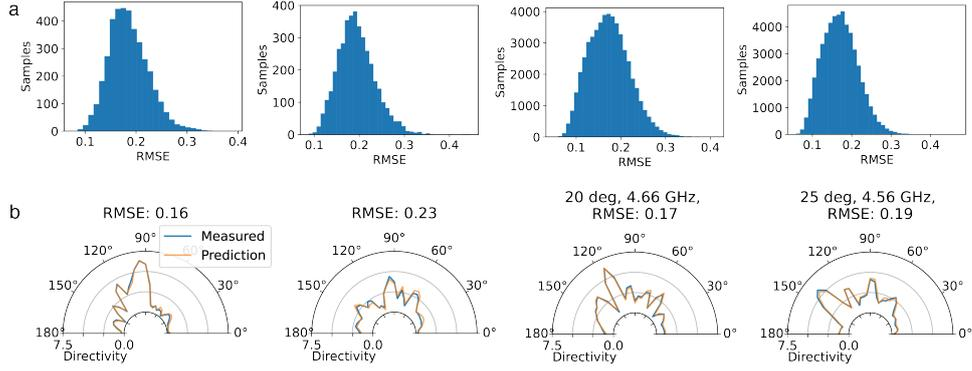
**Extended Data Fig. 2** Performance for the predictor for four cases. (a) RMSE distribution from case A to case D, in the test set. (b) Visual examples with typical error level.
