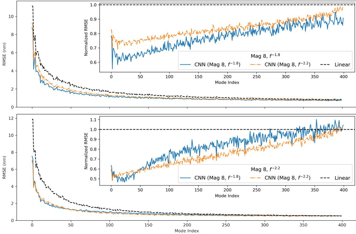
**Fig 11** Two models were trained on different  $f$ -values and testing was performed on both sets of data. The main figures show the error against the true modal coefficient. The insert figures show error relative to the linear baseline.
