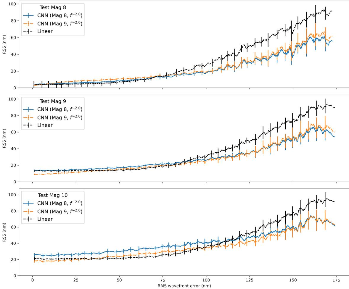
**Fig 8** Model reconstruction quality as a function of RMS for magnitudes 8, 9, and 10. Models were trained on either magnitude 8 or 9 data following a  $p = -2$  power law. Moving averages are plotted to help visualize the trend, with error bars showing one standard deviation for that window.
