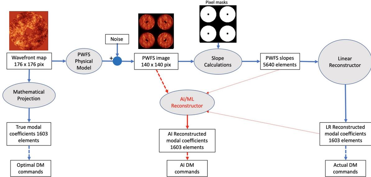
**Fig 1** Outline of the simulation pipeline. Thin red dotted lines are possible inputs to the ML model that we did not pursue in this work. The thick red lines show the inputs and outputs of the proposed ML model.
