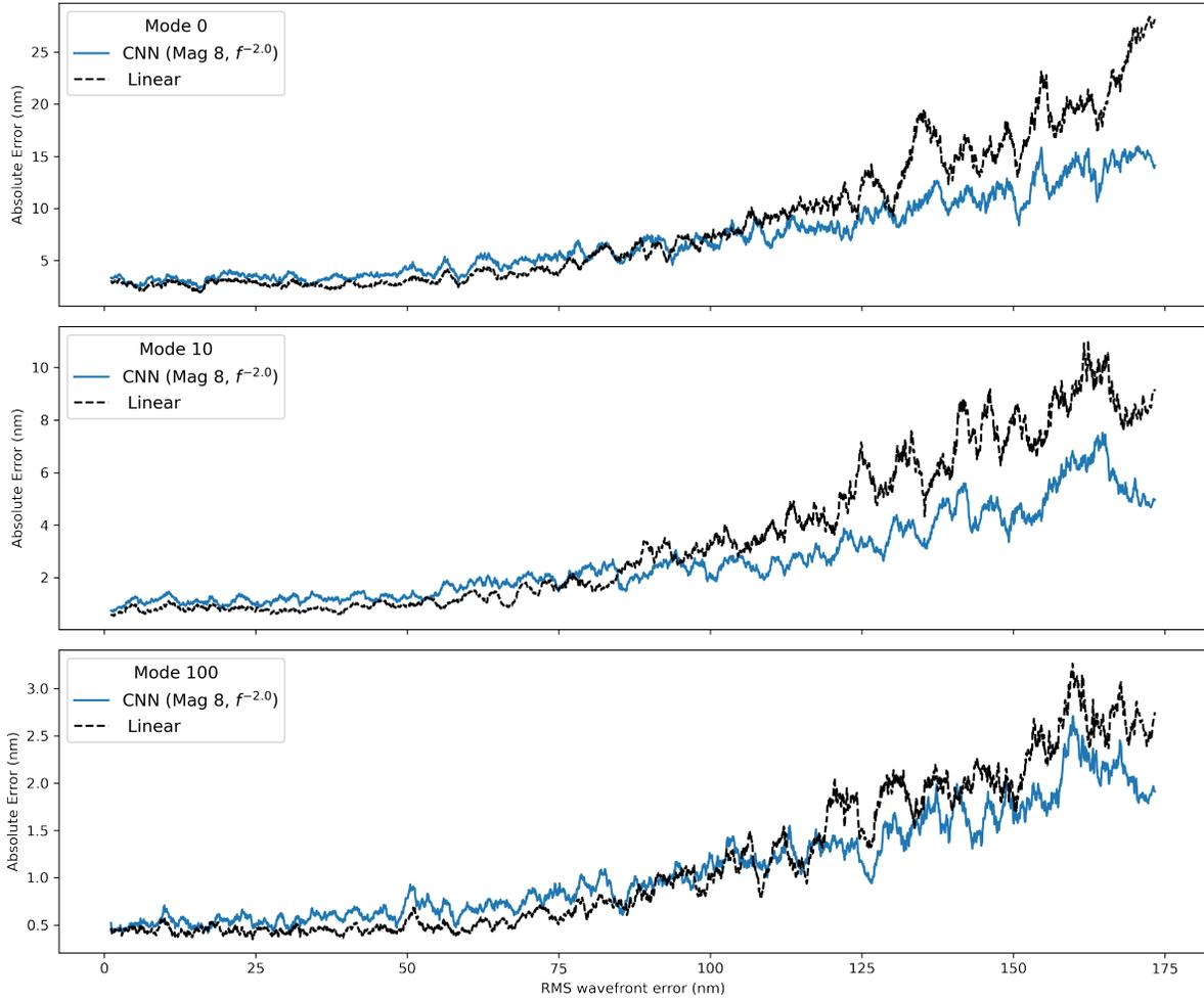
**Fig 9** A selection of three modes showing reconstruction quality by RMS on magnitude 8 samples. Moving averages are plotted to help visualize the trend.
