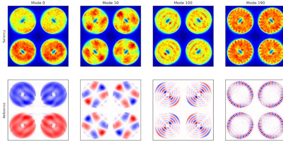
**Fig 10** A selection of modes comparing saliency and idealized Karhunen—Loève modes. The top row shows the importance of each pixel to the model when determining the modal output. The bottom row shows the corresponding Karhunen—Loève mode.
