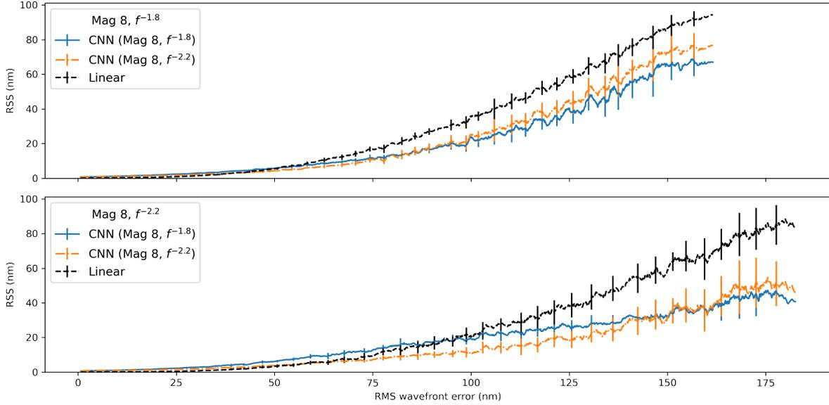
**Fig 12** The error by RMS of two models trained on different  $f$ -values. The upper panel shows models reconstructing  $f^{-1.8}$  samples and the lower reconstructing  $f^{-2.2}$  samples. Moving averages are plotted to help visualize the trend. Error bars are one standard deviation for that window.
