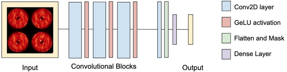
**Fig 4** Our proposed architecture has three convolutional blocks, followed by flattening and modal reconstruction. The input is a pupil image sample following the reduced intensity preprocessing and the output are the first 400 modes.
