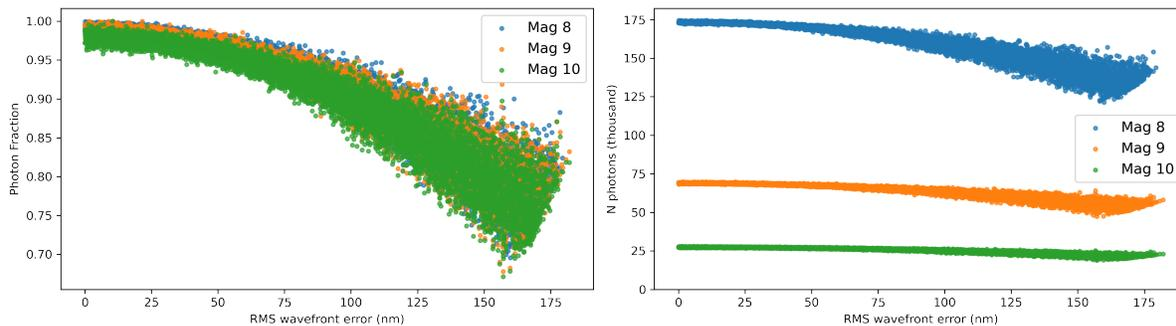
**Fig 2** Flux in the geometric pupil images as a function of the wavefront amplitude for  $p=2$  and various magnitudes. Left: expressed as a fraction of the total number of photons hitting the pupil. This is normalized to the sample with the maximum number of photons for each magnitude. Right: expressed in absolute number of photons.
