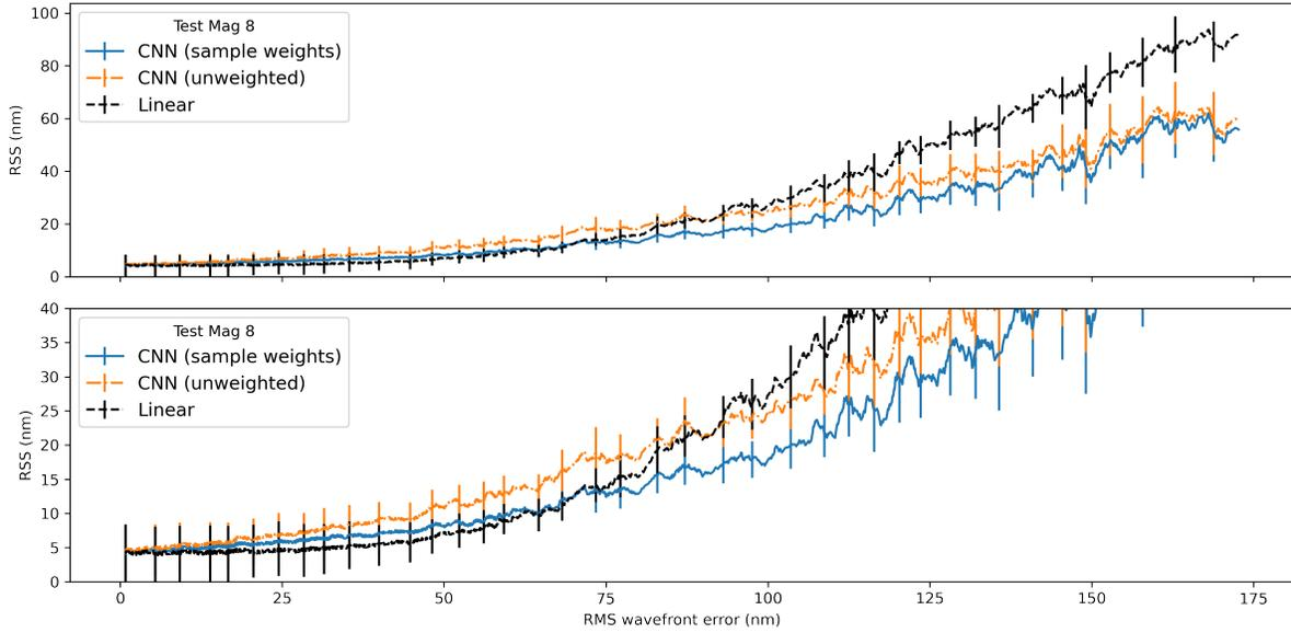
**Fig 5** Weighting samples by RMS value improves model performance. The top panel shows the overall change, and the lower panel shows a zoomed-in view of the lower ( $< 125\text{nm}$ ) RMS cases. Samples were weighted based on their RMS, with low RMS samples being higher weighted. Moving averages are plotted to help visualize the trend, and error bars are the standard deviation of the window.
