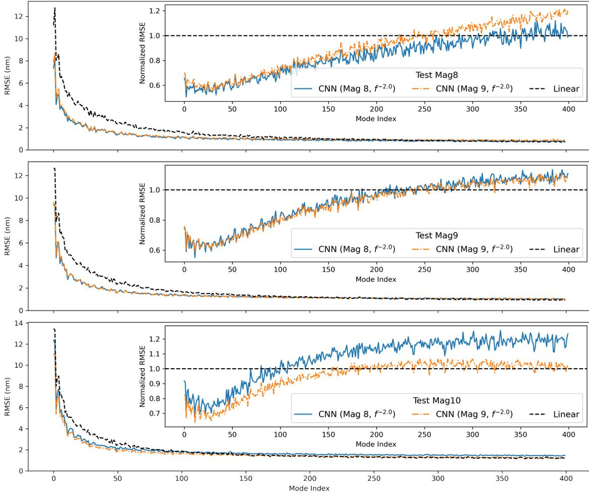
**Fig 7** The error by mode of the best proposed model on three guide stars of different magnitudes. The main panels show the CNN outperforms the linear model at lower modes. Inset panels show reconstruction change relative to the linear baseline.
