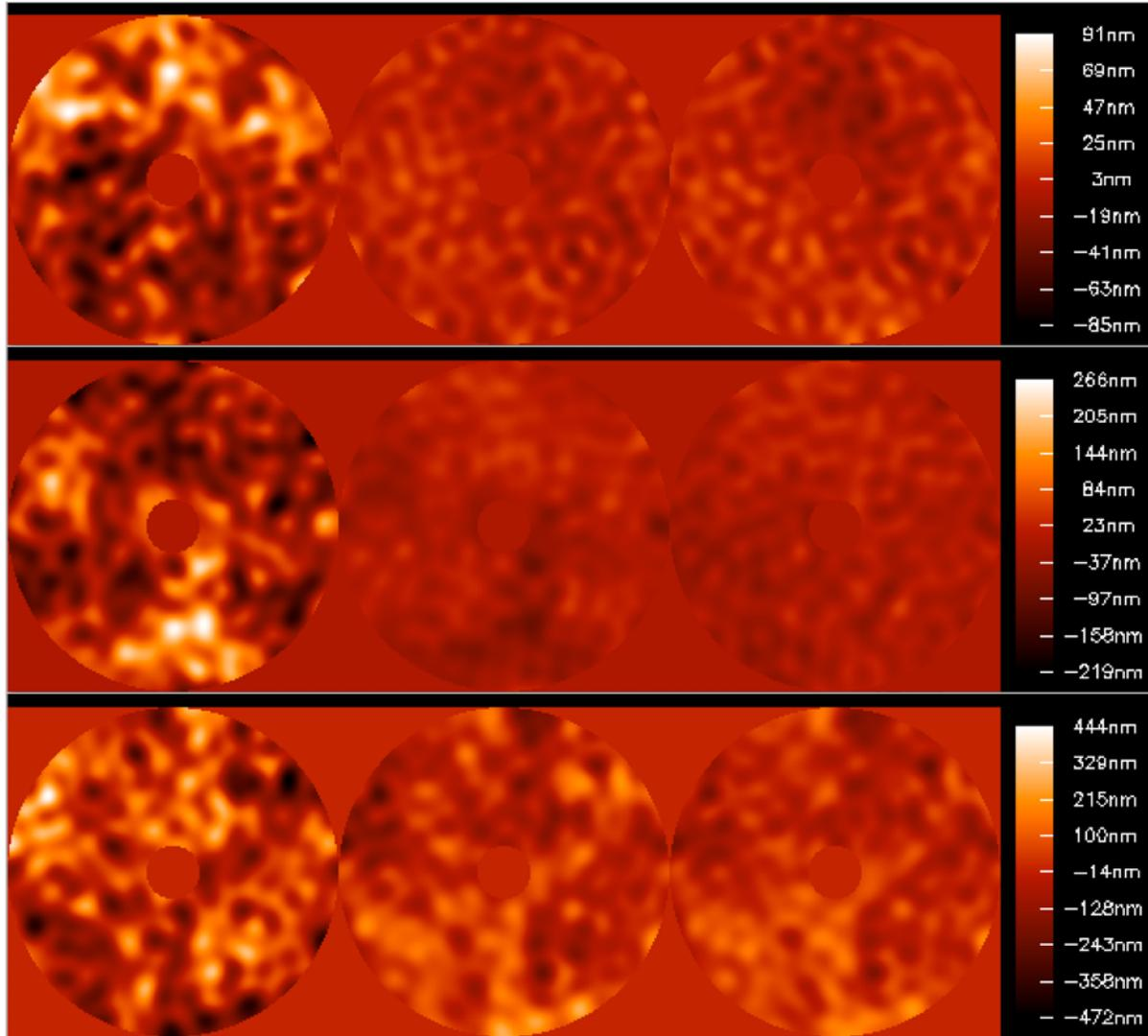
**Fig 6** Left: Incoming wavefront map, 400 KL modes (30/80/134 nm RMS). Middle: residual wavefront error map after linear reconstruction (8/25/85 nm RMS). Right: residual wavefront error map after CNN reconstruction (10/19/69 nm RMS).
