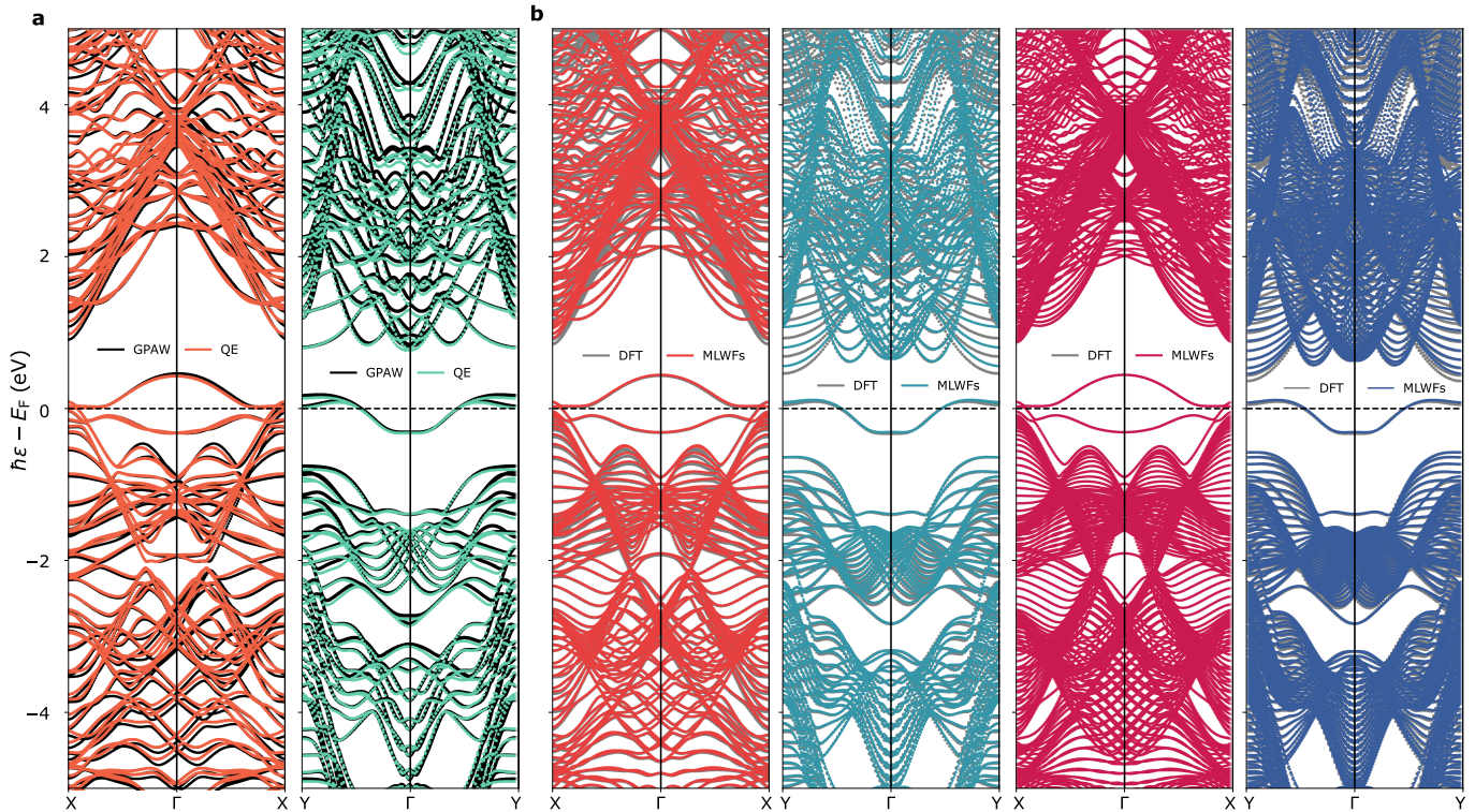
FIG. S1. Electronic band structure in phosphorene nanoribbons. The Wannier tight-binding (WTB) Hamiltonians are constructed from ab-initio electronic band structure calculations performed using the Quantum Espresso (QE) code [1], which forms the basis for optical response calculations performed at the level of the random-phase approximation (RPA). In Fig. 1 of the main text we compare the linear optical response obtained from WTB-RPA simulations with that obtained directly from the GPAW code [2, 3], from which the electronic band structure is computed independently from first-principles for the smallest armchair (AC) and zigzag (ZZ) phosphorene nanoribbons (PNRs) considered. In panel a we present the electronic band structures of the smallest PNRs considered in the main text, as obtained using GPAW (black curves) and QE (colored curves) codes for AC and ZZ ribbons of indicated widths W . Panel b shows the band structures obtained directly from QE for larger ribbons (black curves), which are reproduced by the bands obtained upon diagonalization of the constructed WTB Hamiltonian.
