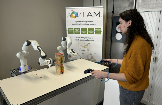
Fig. 2: Depiction of the teleoperation procedure, where a user uses the VIVE handheld controller devices to prescribe a reference for both end effectors.
