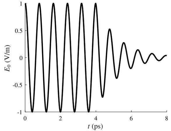
Fig. 4. The time-domain excitation pulse of the incident plane-wave in MEEP.
