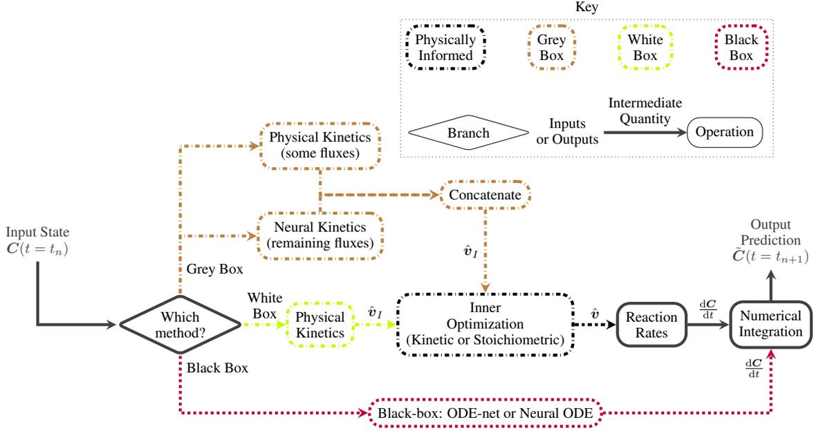
Figure 1: **White, gray, and black inner architectures.** Operations are boxed, data or predictions are unboxed, and notable named intermediates are labeled on edges. Color and pattern are used to distinguish between model pathways that are distinct between the gray-, white-, and black-box approaches, or common to all three.
