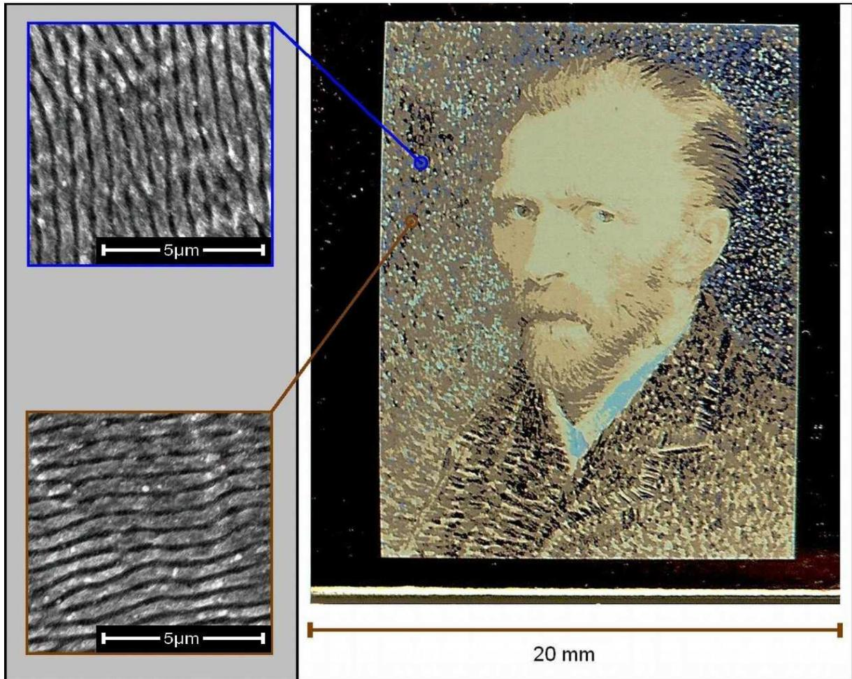
Fig. 7: Photograph (right) of a polished 316L stainless steel sample after fs-laser processing [800 nm, 150 fs, 5 kHz] of a miniaturized self-portrait of the painter Vincent van Gogh. The insets (left) are top-view scanning electron micrographs of LSLF with two different local orientations. (Reprinted with permission from [Dusser, 2010], © Optical Society of America).
