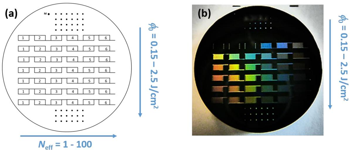
Fig. 6: (a) Scheme of laser processing. (b) Photograph of a polished 100Cr6 steel sample (24 mm diameter) after fs-laser processing [800 nm, 30 fs, 1 kHz] of spots, lines, and areas. The colors arise from optical diffraction of ambient light at laser generated LSFL. (© 2016 IEEE. Reprinted, with permission, from [Bonse, 2017], Bonse, J., et al., Laser-induced periodic surface structures—A scientific evergreen, IEEE J. Sel. Top. Quantum Electron, 2017, 23:9000615).
