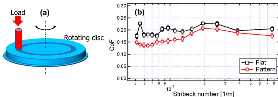
Fig. 26: (a) Scheme of pin-on-disk tribological test. (b) Stribeck curve of LIPSS (LSFL, referred to as “pattern”) on stainless steel along with a reference curve for a polished (flat) surface. (Reprinted from [Gnilitskyi, 2019] Gnilitskyi et al., Tribological Properties of High-Speed Uniform Femtosecond Laser Patterning on Stainless Steel, Lubricants (Basel, Switzerland) **7**:83, Copyright 2019 under Creative Commons BY 4.0 license. Retrieved from <https://doi.org/10.3390/lubricants7100083>).
