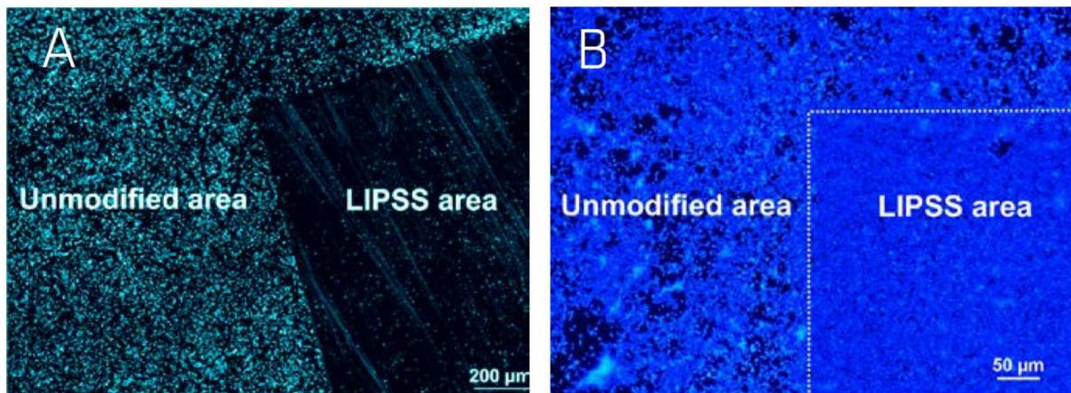
Fig. 19: Fluorescence microscope images of steel samples (V4A), partially processed with LSFL and subsequently colonized with dye-stained (a) *E. coli* bacteria after incubating of 18h and (b) *S. aureus* bacteria after incubating of 20h. (Reprinted from [Epperlein, 2017], Appl. Surf. Sci., Vol. **418**, Epperlein et al., Influence of femtosecond laser produced nanostructures on biofilm growth on steel, 420–424, Copyright (2017), with permission from Elsevier).
