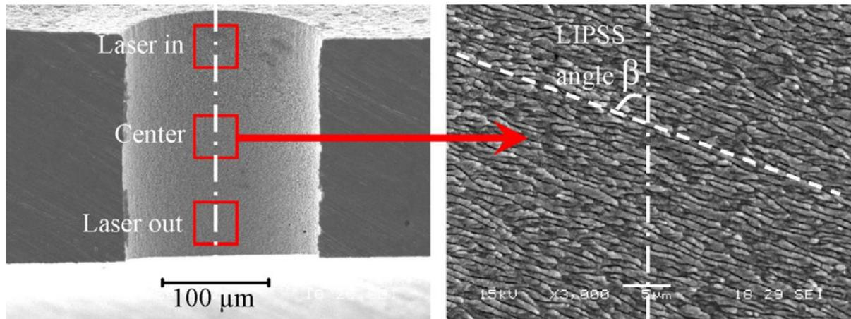
Fig. 34: SEM micrographs of a cross-section of a fs-laser drilled spray hole (left) and the magnified nanostructures in the center of the surface of the spray hole (right). (Reprinted from [Romoli, 2014], CIRP Annals, Vol. 63, Romoli, et al., Ultrashort pulsed laser drilling and surface structuring of microholes in stainless steels, 229–232, Copyright (2014), with permission from CIRP).
