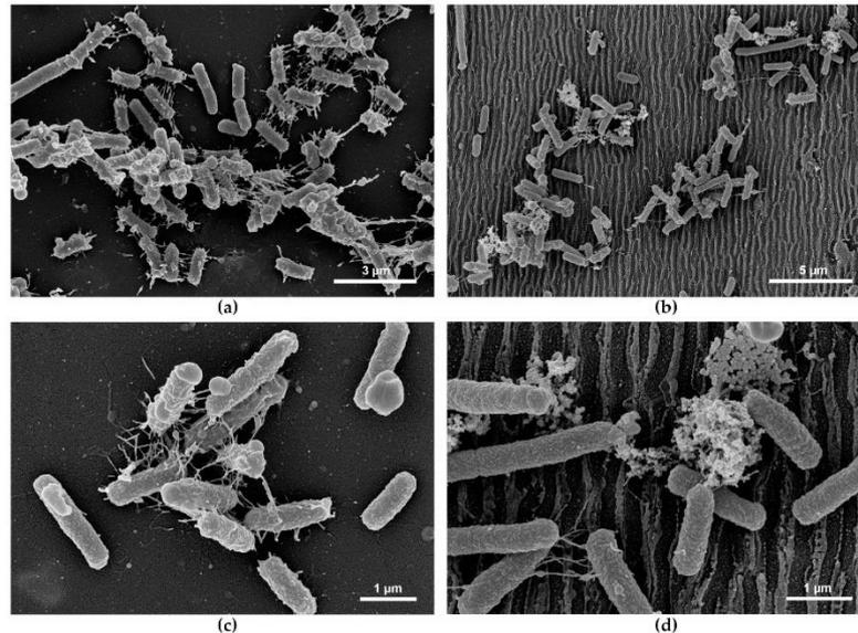
Fig. 21: SEM micrographs of *E. coli* bacteria on (a,c) non-irradiated (flat) PET and (b,d) laser-structured PET covered with LSFL of < 300 nm spatial period. Note the different scale bars. (Reprinted from [Richter, 2021], Richter et al., Spatial Period of Laser-Induced Surface Nanoripples on PET Determines *Escherichia coli* Repellence. *Nanomaterials* **11**:3000 (2021), Copyright 2021 under Creative Commons BY 4.0 license. Retrieved from <https://doi.org/10.3390/nano11113000>)
