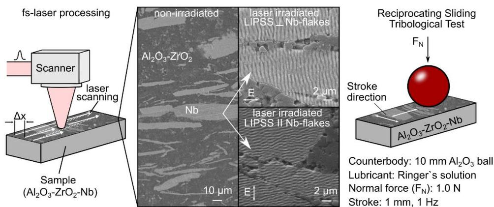
Fig. 24: Scheme of fs-laser processing and reciprocating sliding tribological tests (RSTT) on selectively LIPSS-structured  $\text{Al}_2\text{O}_3\text{-ZrO}_2\text{-Nb}$  composites. (Reprinted from [Kunz, 2020], *Appl. Surf. Sci.*, Vol. **499**, Kunz et al., Tribological performance of metal-reinforced ceramic composites selectively structured with femtosecond laser-induced periodic surface structures, 143917, Copyright (2019), with permission from Elsevier).
