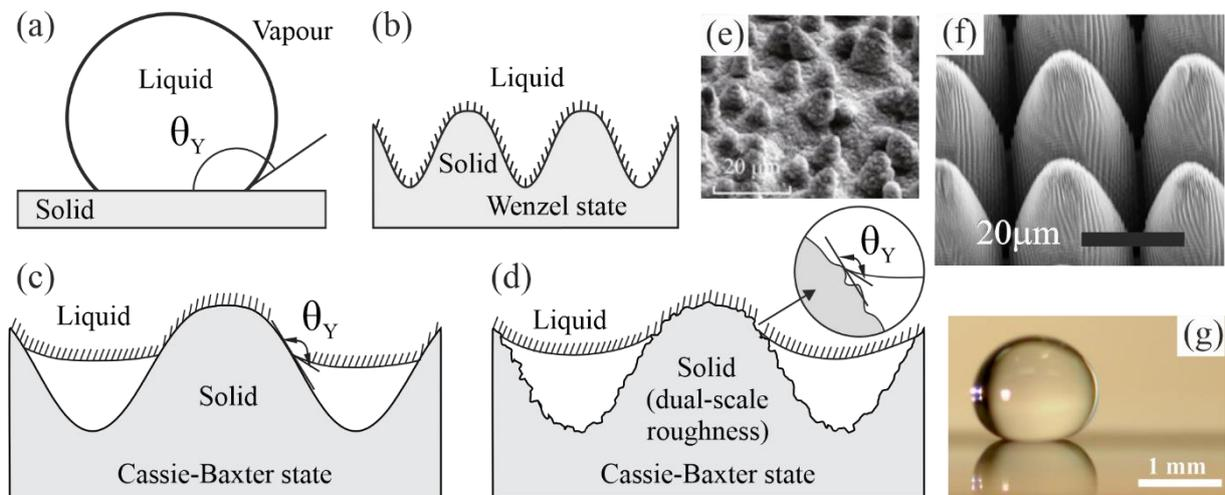
Fig. 10: (a) Definition of contact angle  $\theta_Y$  [°] of a liquid (droplet) resting on a flat solid in a gaseous environment (solid–liquid–vapour system). (b) Wenzel state, in which the liquid fully wets the surface (c) Cassie-Baxter state, in which air is trapped below the liquid. (d) Liquid on a hierarchical (here dual-scale) surface topology composed of micrometer and nanometer scale surface roughness, resulting in increased Apparent Contact Angle
