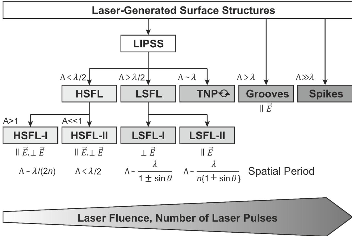
Fig. 4: Classification of laser-generated surface structures. Adapted from [Mezera, 2020].
