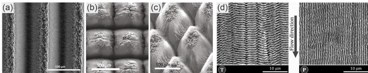
Fig. 16: (a)-(c) SEM micrographs of various multiscale surface morphologies for liquid drag reduction, consisting of micrometer scaled patterns superimposed by LIPSS on the slide walls and nanoparticles on the peaks. (d) SEM micrographs of LSFL on mould steel aiming a drag reduction in polymer injection moulding.
