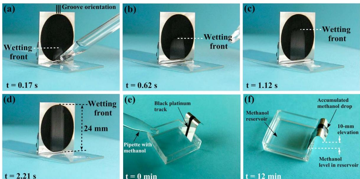
Fig. 13: (a)-(d) Photographs showing the methanol transport against gravity on a vertically standing laser-processed black platinum surface. (e)-(f) Photographs showing the vertical transport of methanol and liquid
