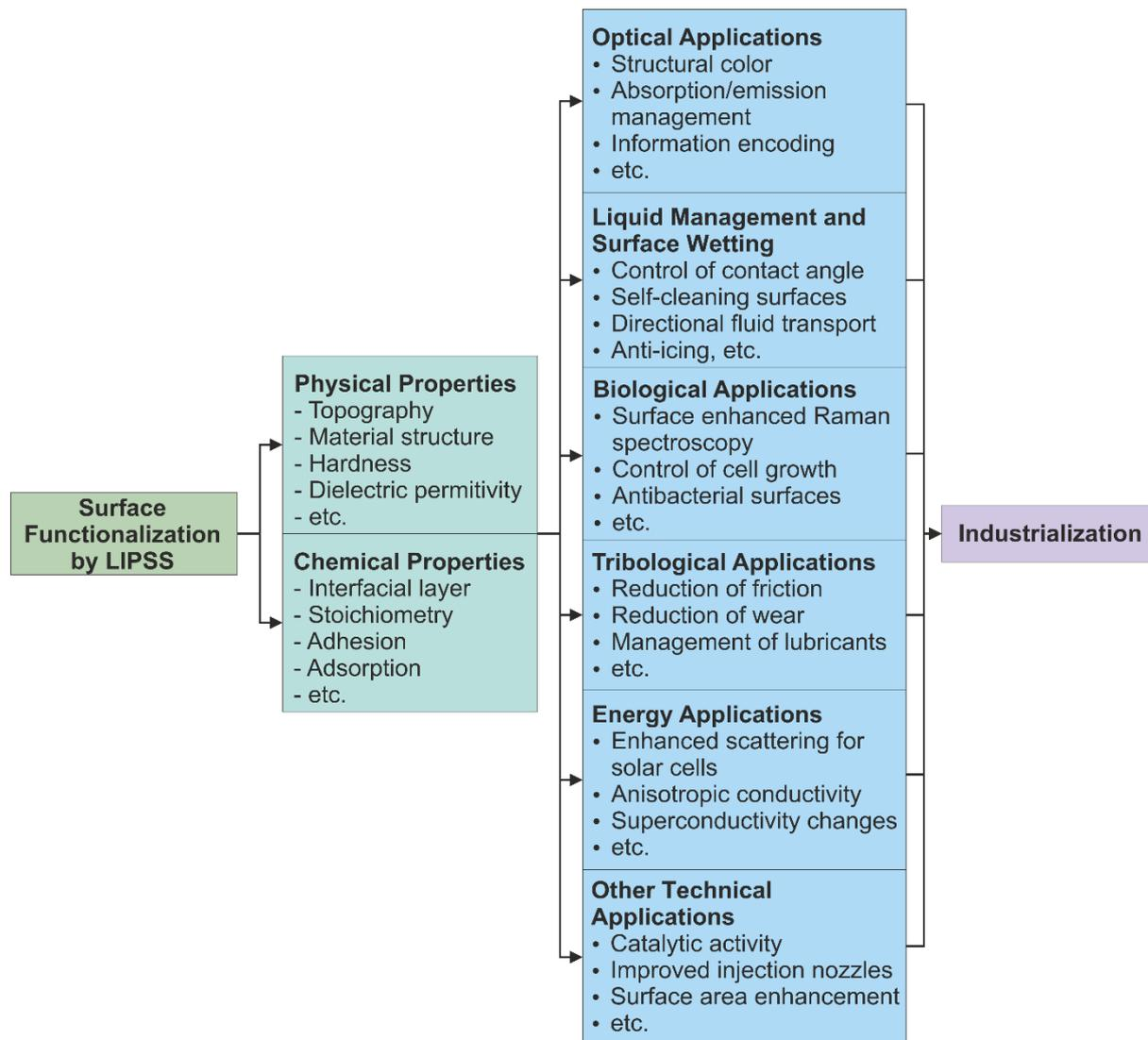
Fig. 5: Scheme of properties affected by LIPSS and resulting applications for surface functionalization, providing the frame for this book chapter. Inspired by [Florian, 2020a].
