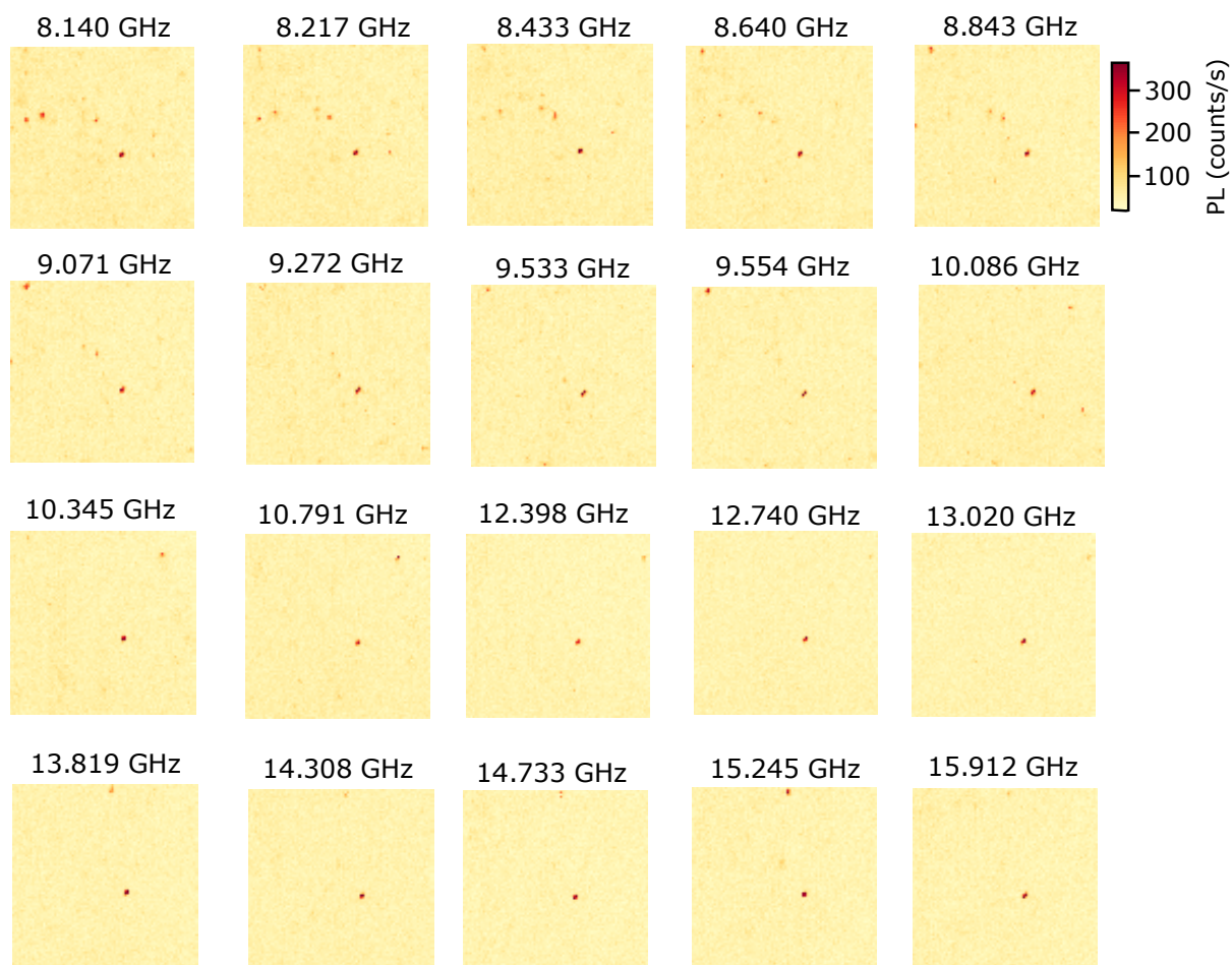
Supplementary Figure S13. PLE maps, sample B - natural abundance of isotopes (excitation laser frequency range: 8 to 16 GHz). Photoluminescence maps for different detunings of the excitation laser for the sample with natural abundance of Si and C isotopes. Each map shows a 30 \mu\text{m} by 30 \mu\text{m} area. A PL spot is visible around the centre of all maps: its PLE spectrum is very broad and not associated to a V centre. For these measurements, we use an integration time of 1 s per step, an excitation power of 14 \mu\text{W} for the repump laser, and 4 \mu\text{W} for the telecom laser.
