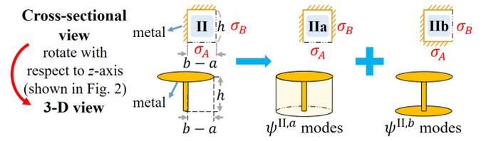
Fig. 3. An illustration of the resonator method [17], [21] used to expand the fields in region II.
