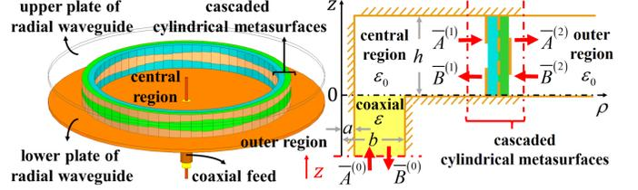
Fig. 1. Perspective and cross-sectional (a constant  $\phi$  plane in cylindrical coordinates) views of cascaded cylindrical metasurfaces excited by a coaxial feed. The inner conductor of the feed touches the upper plate of the waveguide.
