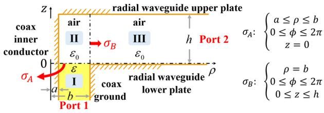
Fig. 2. A coaxial cable to radial waveguide junction. The junction is rotationally symmetric with respect to the  $z$ -axis, and is divided into three regions. The interface between region I (dielectric filled) and region II is  $\sigma_A$ , while the interface between regions II and III is  $\sigma_B$ .
