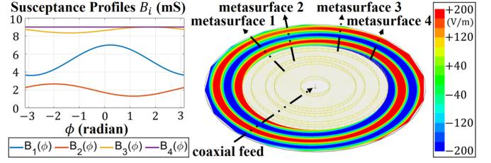
Fig. 4. The synthesized susceptance for each metasurface layer. Admittance  $Y_i(\phi) = jB_i(\phi)$ . The real part of the  $E_z$  field in the outer region (obtained through full-wave simulation) is also shown.
