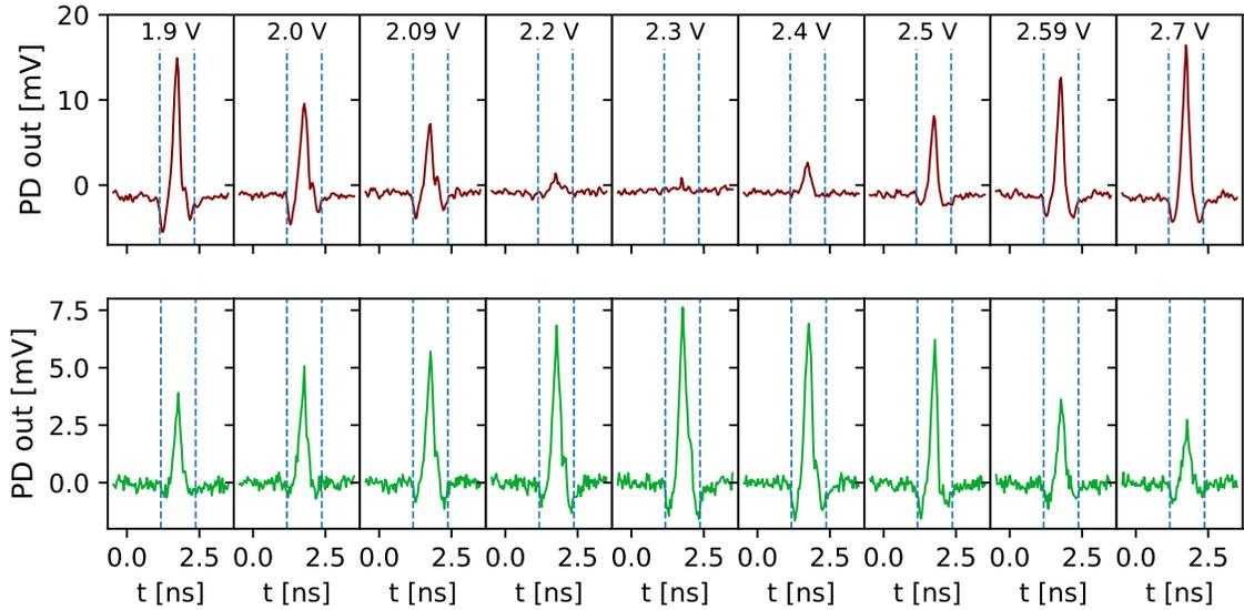
Figure 4: Demonstration of spike amplitude weighting at both THRU (top row) and DROP (bottom row) ports of the micro-ring resonator output. In each case, the spike trace shown corresponds to a mean spike envelope calculated from all the recorded repetitions for a given value of  $V_{MR}$ .
