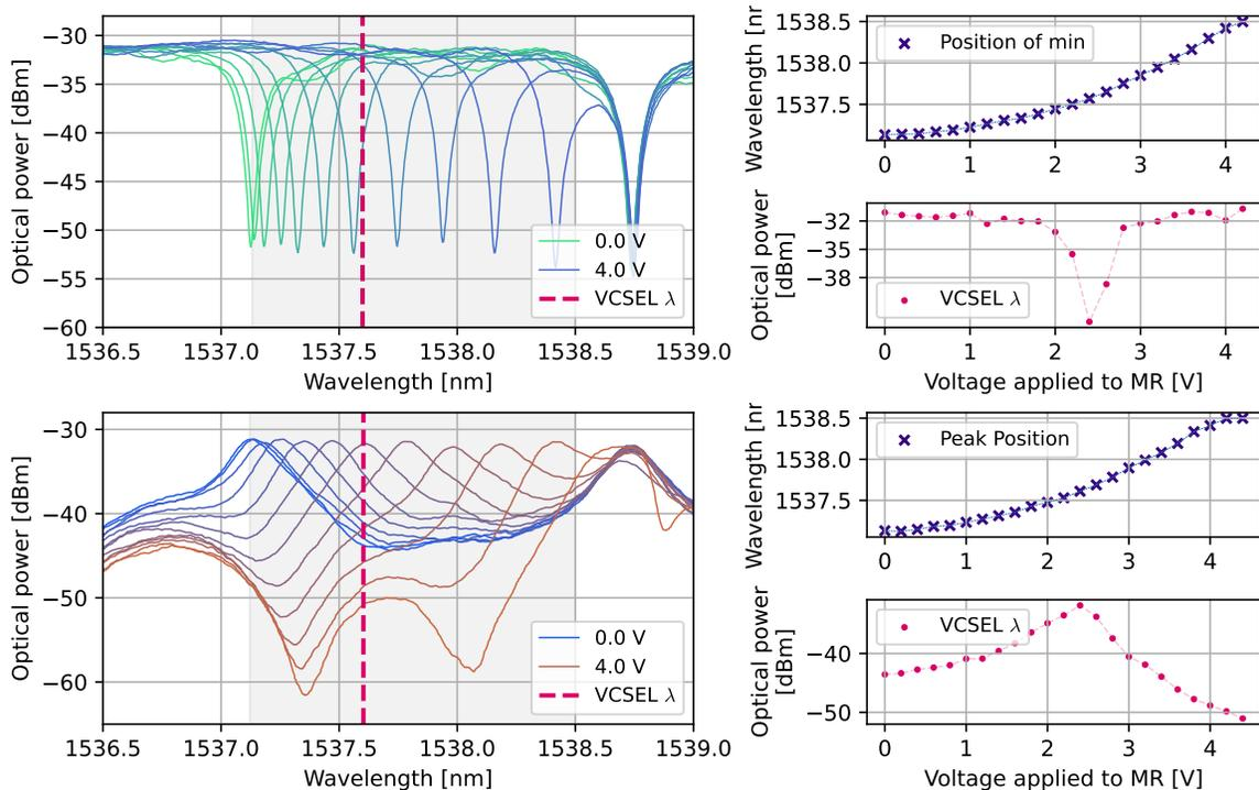
Figure 2: micro-ring characterization: THRU port readout (top) and DROP port readout (bottom), with power at fixed wavelength (dashed line) and maxima (minima) position as function of  $V_{MR}$ .
