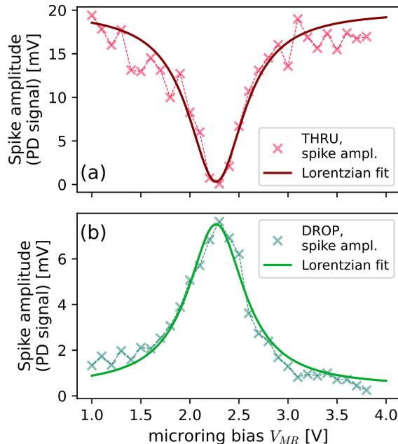
Figure 5: Mean amplitudes of all spikes ( $n_s = 7$  per measurement,  $n_m = 15$  repetitions) as a function of micro-ring heater bias  $V_{MR}$  with Lorentzian fit (solid line) using the least squares method. The two plots show (a) THRU; (b) DROP port readouts.
