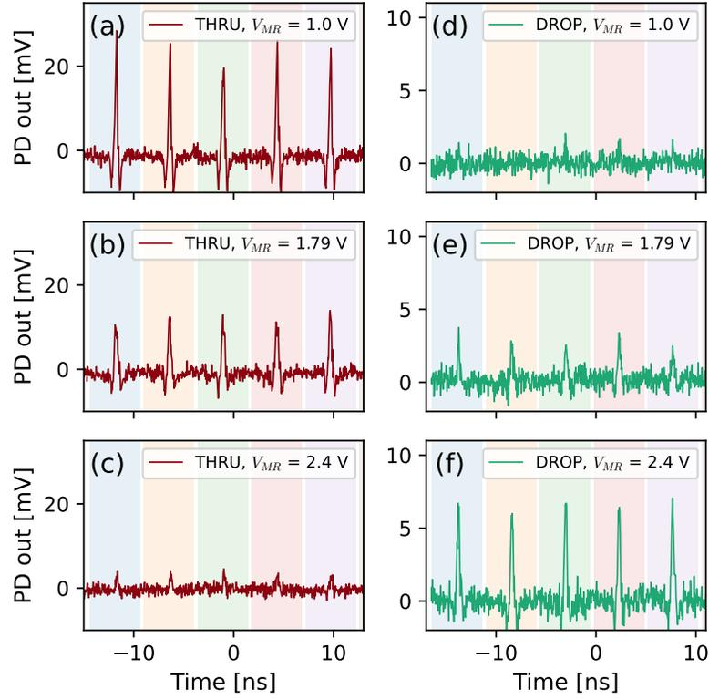
Figure 3: Sequences of deterministically triggered excitable spikes in the VCSEL-neuron after passing through the weighting micro-ring for three different values of  $V_{MR}$ . Traces were recorded on both outputs of the micro-ring: the THRU port (left column, in red) and the DROP port (right column, in green).
