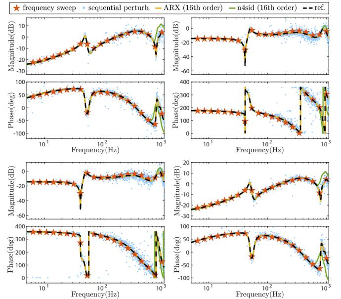
Fig. 7: Bode diagrams of the identified  $2 \times 2$  grid impedance  $Z_g(s)$  in Fig. 6 using different parametric and nonparametric identification methods. The black dashed line indicates the analytically computed true grid impedance.
