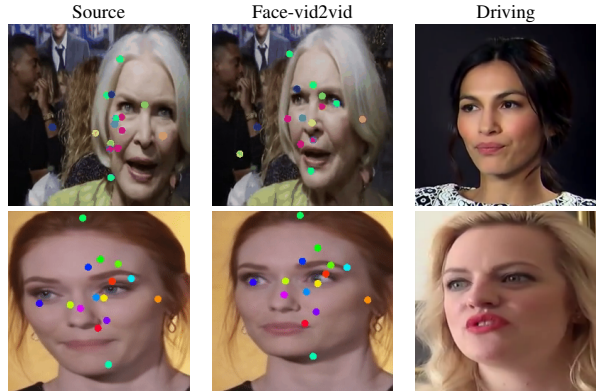
Figure 1: Problems of existing keypoint-based talking-head method. Despite its superior performance and compact representation, we observe two common problems stem from the keypoint design. First, the keypoints may fail to establish correct correspondence between source and driving frame especially when the head poses are significantly different, which leads to incorrect reconstruction. Second, the keypoints are not dense enough around semantically important regions like the mouth, so the model fails to transfer fine-grained expression or motion.
