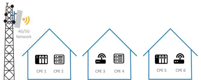
Fig. 1. Illustration of Fixed Wireless Network (FWA), where the BS serves various CPEs at home with fixed-location. CPE: customer premise equipment.
