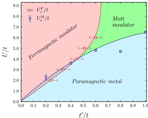
FIG. 7. Phase diagram of the Hubbard model on the anisotropic kagome lattice at half-filling. Critical points labelled  $U_c^F/t$  and  $U_c^M/t$  have been determined through data in Fig. 4 and Fig. 6(e), respectively; see text. The dashed lines through the critical points are guides to the eye.
