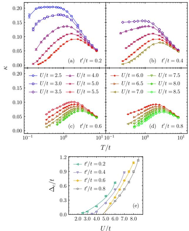
FIG. 6. Panels (a)-(d): Compressibility as a function of temperature, for fixed values of  $t'/t$ , and different values of  $U/t$ . (e) Estimates of the gap obtained by fitting an exponential form,  $\kappa \propto \exp(-\Delta_c/k_B T)$ , to the low temperature data of panels (a)-(d); see text. When not shown, error bars are smaller than the symbol size, while the lines are parabolic fits to the curves.
