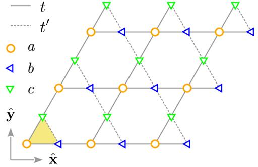
FIG. 1. The kagome lattice is composed of hexagons tiled with intervening corner-sharing triangles; points  $a$ ,  $b$  and  $c$  comprise the unit cell (highlighted triangle). Solid and dashed lines indicate hopping amplitudes  $t$  and  $t'$ , respectively.
