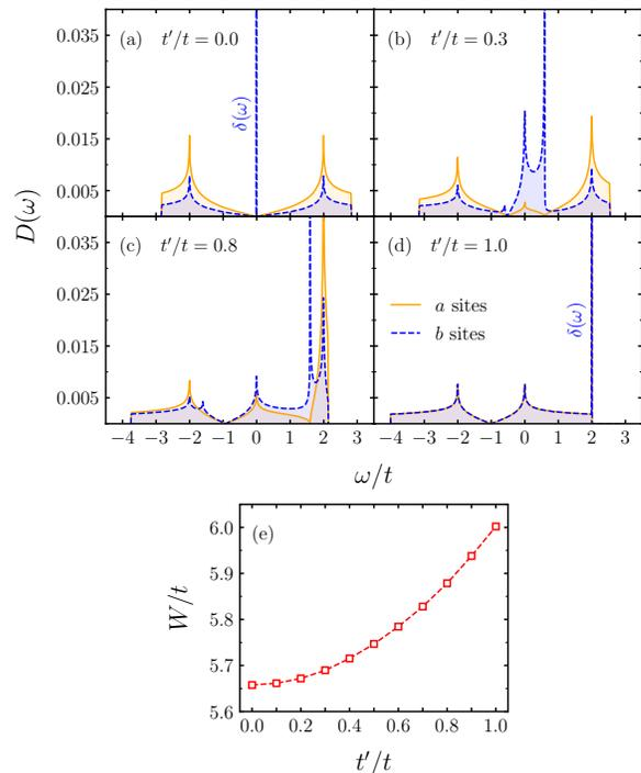
FIG. 2. (a)-(d): Site-resolved non-interacting DOS for tight-binding fermions on a kagome lattice for different values of  $t'/t$ , the ratio between hoppings along  $bc$  sites and along sites involving  $a$  sites (see Fig. 1);  $\hbar\omega$  is measured relative to the Fermi energy for half filling. (e): Bandwidth,  $W/t$ , as a function of  $t'/t$ ; the dashed line is a guide to the eye.
