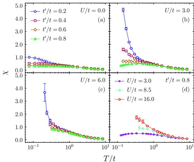
FIG. 5. Temperature dependence of the uniform susceptibility in linear-log plots. Each of the panels (a) to (c) shows data for fixed  $U/t$  and different  $t'/t$ ; panel (d) shows data for fixed  $t'/t = 0.8$ , and different values of  $U/t$ . Data have been obtained for  $L = 6$ , except in (a), in which case  $L = 18$  was used. When not shown, error bars are smaller than the data points.
