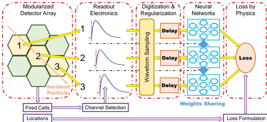
Figure 1: The system diagram of the proposed method based on the conventional nuclear detector dataflow. The modularized detector array front end provides information of fired cells and their locations for readout electronics to select valid channels and for the training back end to construct physics-constrained formulation of the loss function.
