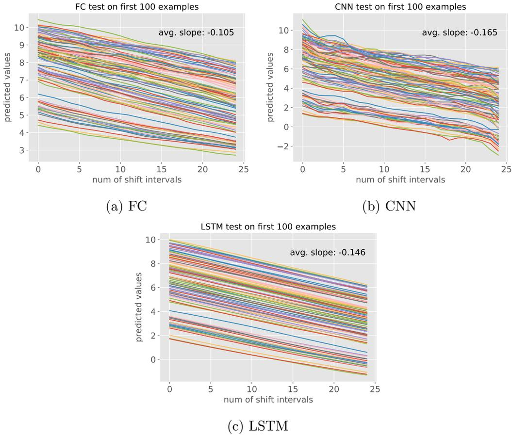
Figure 7: Demonstration of the calibration process (showing only the first 100 examples) with equidistantly shifted waveform samples for the NN models: (a) Fully-connected network; (b) Convolutional neural network; (c) Recurrent neural network with long short-term memory.
