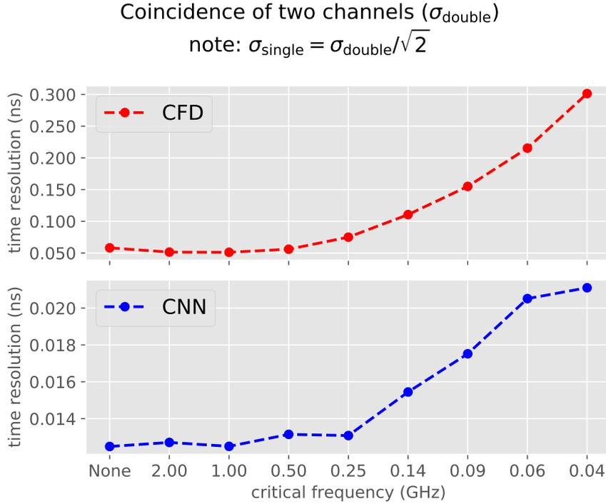
Figure 4: Comparison of digital constant fraction discrimination (CFD) and convolution neural network (CNN). The time resolution is the standard deviation of timing differences, plotted versus variable critical frequencies of low-pass filters.
