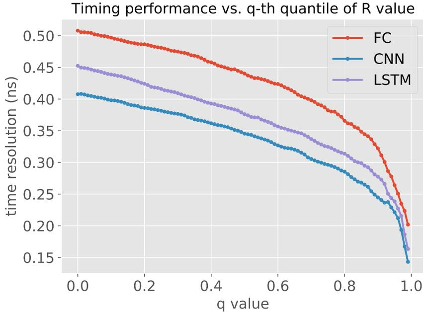
Figure 9: Comparison of timing performance of NN models at different q-th quantiles of the R value.
