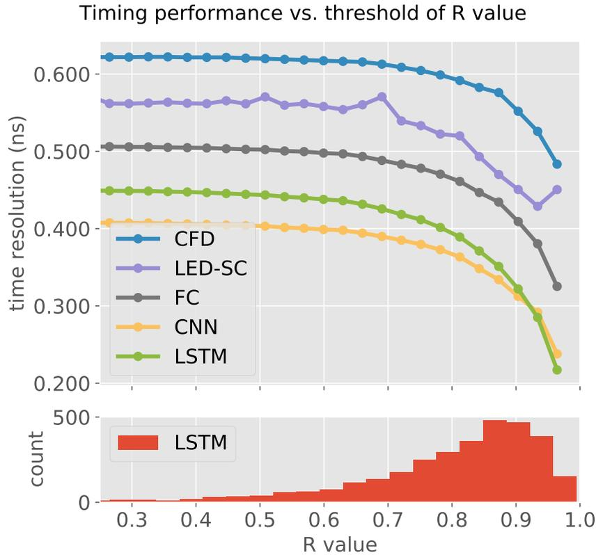
Figure 10: The lower histogram shows the distribution of the R value with the LSTM model. Based on the histogram, the upper plot shows the timing performance of two traditional methods (digital constant fraction discrimination and leading edge discrimination with slewing correction) and also NNs at different R value thresholds.
