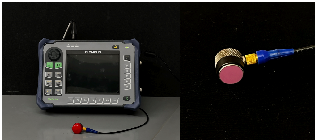
Figure 7: The Olympus Epoch 650 Ultrasound NDT Flaw Detector used in this study (left). The transducer has a 12.7 mm diameter and is a straight beam single element transducer (right).
