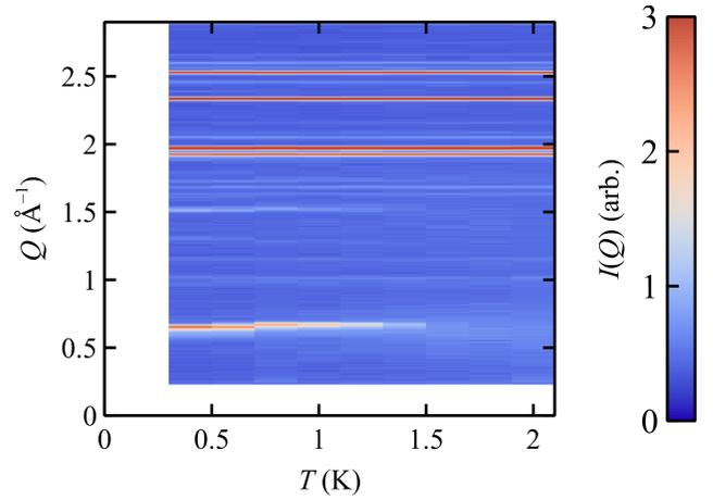
Figure 3. Overview of neutron-diffraction data, showing diffraction intensity in false color as a function of temperature  $T$  and wavevector  $Q$ . Magnetic ordering at  $T_{N1} \approx 1.6$  K is indicated by the appearance of new (magnetic) Bragg peaks, and the magnetic phase transition at  $T_{N2} \approx 0.6$  K is indicated by a change in position of these peaks. Nuclear peaks, such as the four intense peaks at  $Q > 1.8 \text{ \AA}^{-1}$ , do not change position with temperature.
