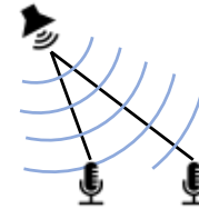
Fig. 3. Illustration of the phase difference in different microphones of a beamforming array.
