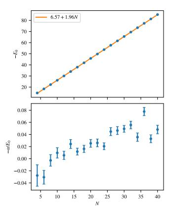
FIG. 21. Scaling of systematic  $\Delta_{\tau}$  error for L=4,  $\Theta=2$ , and S=1/2. For each point, we simulated with a range of different values for  $\Delta \tau$  and fitted the energy to  $E(\Delta_{\tau})=E_0+\alpha {\Delta_{\tau}}^2$ .
