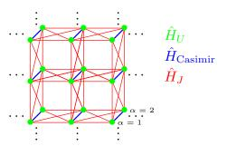
FIG. 4. Sketch of the structure of the QMC Hamiltonian for 2S=2.  $\hat{H}_U$ : Hubbard term for freezing out charge degrees of freedom.  $\hat{H}_{\text{Casimir}}$ : Term for maximizing the eigenvalue of the Casimir operator.  $\hat{H}_J$ : Antiferromagnetic interaction between elemental spins.
