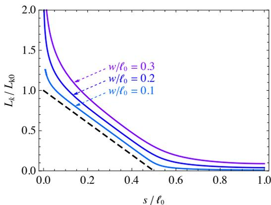
FIG. 3. Kinetic inductance  $L_k$  vs turn width  $s$  for  $w/\ell_0 = 0.1, 0.2$ , and  $0.3$ . The dashed line corresponds to the limit of  $w/\ell_0 \rightarrow 0$ ,  $L_k = \mu_0 \lambda^2 (\ell_0 - 2s) / (wd)$ .  $L_k$  and  $s$  are normalized by  $L_{k0}$  from Eq. (2) and  $\ell_0$ , respectively.
