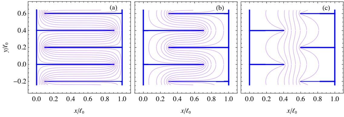
FIG. 2. Streamlines of the current density in meander superconducting nanostrips of  $w/\ell_0 = 0.2$  for (a)  $s/\ell_0 = 0.1$  ( $s < w$ ), (b)  $s/\ell_0 = 0.3$  ( $w < s < \ell_0/2$ ), and (c)  $s/\ell_0 = 0.6$  ( $s > \ell_0/2$ ). Thick lines correspond to the edges of the nanostrips.
