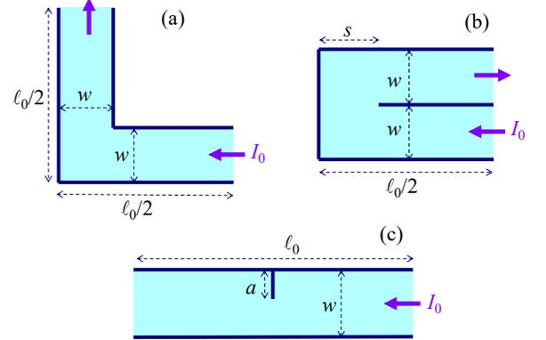
FIG. 4. Superconducting nanostrips of length  $\ell_0$  and width  $w$  with (a) a 90° turn, (b) a 180° turn of turn width  $s$ , and (c) a thin vertical notch of length  $a$ .
