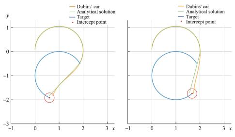
Fig. 13 Comparison of circular intercept trajectories at different initial parameters.
