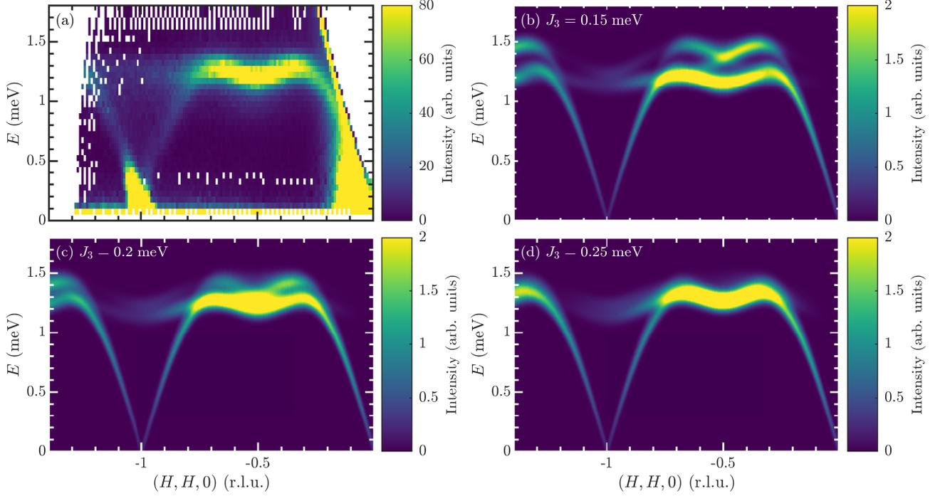
FIG. 15. Spin-wave dispersion along  $(H, H, 0)$  for: (a) MACS single crystal inelastic neutron scattering spectrum. (b)-(d) Inelastic neutron scattering spectrum calculated from linear spin-wave theory by fixing different  $J_3$  values. The other parameters for these calculations are listed in Table V.
