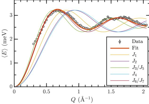
FIG. 14. (data points) First moment computed from the powder data, as a function of the scattering vector amplitude. (red thick curve) First moment calculated from the  $\gamma$  parameters fitted in the single crystal first moment sum rule analysis. (thin curves) Contributions to the first moment from the different exchange paths, normalized to the powder computed first moment.
