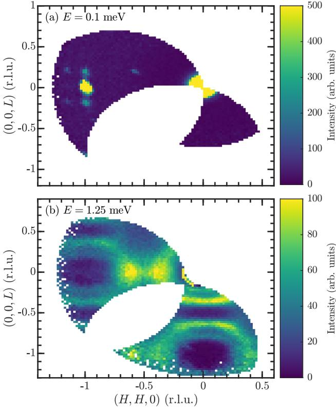
FIG. 6. MACS single crystal inelastic neutron scattering spectra at  $T = 1.4$  K: constant energy slices for (a)  $E = 0.1$  meV and (b)  $E = 1.25$  meV. The weak scattering in (a) at  $(H, H) \sim -0.5$  and displaced at  $(H, H) \sim -1.1$  originate from some crystals miss-aligned by  $\sim 60^\circ$  in the multi crystal mount.
