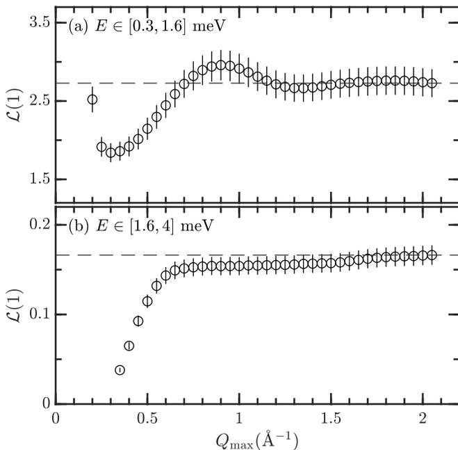
FIG. 9. Integrated intensities as a function of  $Q_{\max}$  the momentum integration upper bound, for (a) one-magnon and (b) two-magnon scattering. The dashed lines indicate the final values for  $Q_{\max} = 2.05 \text{ \AA}^{-1}$ .
