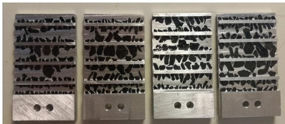
FIG. 3. 1.3 g of single crystals of  $\text{MnSb}_2\text{O}_6$  aligned on four Al plates, and coated with Fomblin oil for inelastic neutron scattering.
