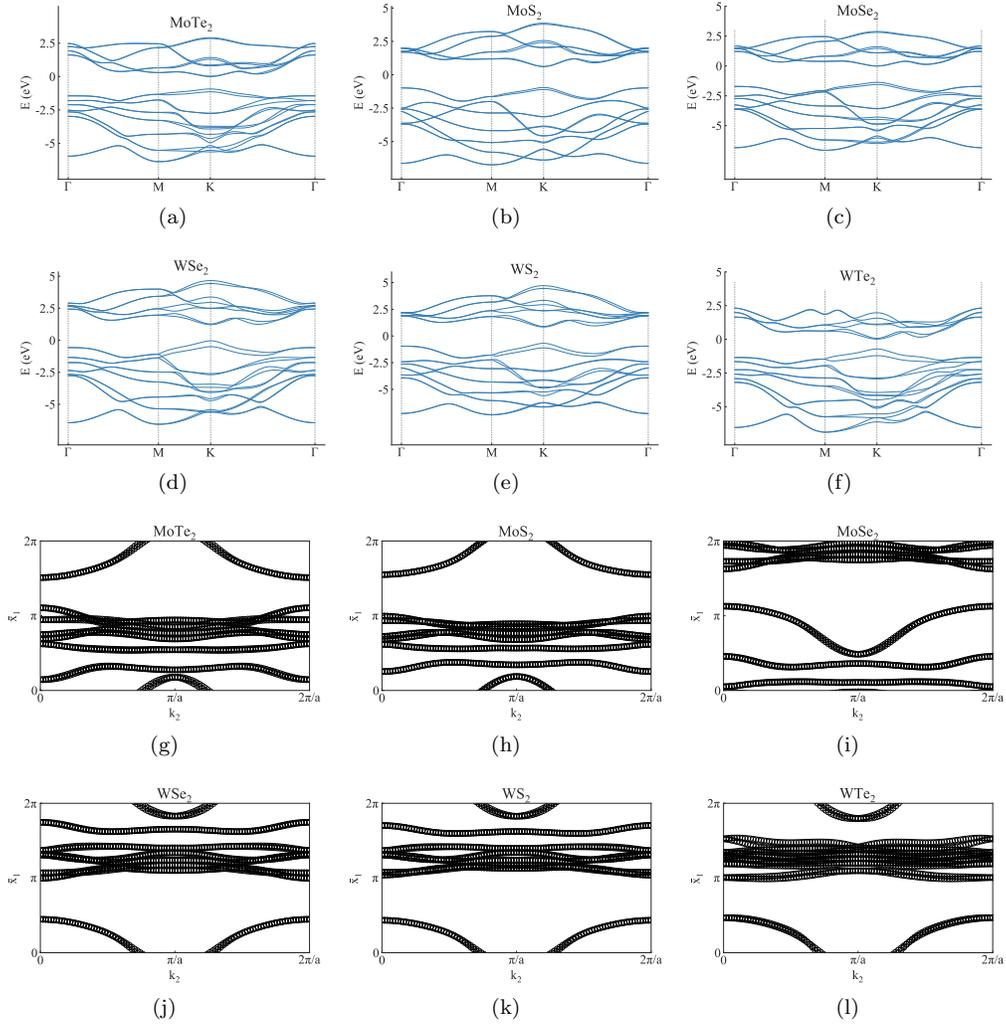
FIG. 9: (a) Bulk band structure along high-symmetry path for 1H-MX<sub>2</sub> TMDs supporting  $|C_{s,G}| = 2$ . (b) Wannier center charge (WCC) spectra in the two-dimensional plane for 1H-MX<sub>2</sub> TMDs admitting ground state spin Chern number,  $|C_{s,G}| = 2$ . In each case the spectra is gapped. As a result, no information about the topological nature of the ground-state can be determined.
