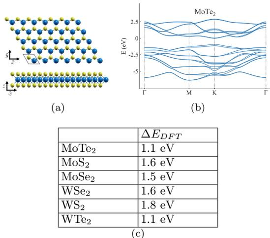
FIG. 2: (a) Structure of 1H-MX<sub>2</sub> phase for two-dimensional transition metal dichalcogenides. Blue atoms indicate transition metal (M), and yellow atoms indicate chalcogen atoms. (b) Bulk band structure along high-symmetry path for 1H-MoTe<sub>2</sub>. (c) Calculated bulk band-gap for materials of interest.
