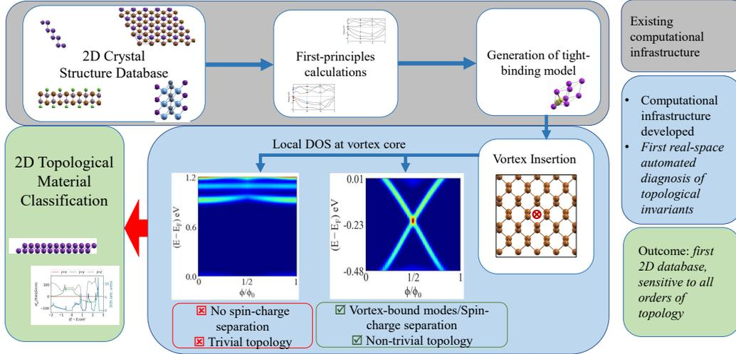
FIG. 1: Diagram detailing work flow for automated identification of bulk topological invariant in 2D materials. Flow ends with plots of local DOS at the inserted vortex core. Examples given are for antimonene (labeled trivial) and bismuthene (labeled non-trivial) in vicinity of the Fermi energy[15]. Bismuthene is non-trivial as we can clearly observe the electromagnetic vortex binding a Kramers pair in the bulk-gap.
