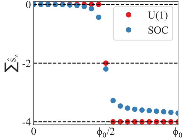
FIG. 8: Spin-expectation value for half-filled system of  $20 \times 20$  lattice sites as a function of flux strength for inserted magnetic vortex in the presence of  $U(1)$  spin-conservation symmetry (denoted  $U(1)$ ) and generic spin-orbit-coupling (denoted SOC), fixing  $t_{3,4} = 0$  and  $t_{3,4} = 1$  respectively in eq. (2). The results demonstrate that the flux tube continues to serve as a spin-pump in the absence of  $U(1)$  symmetry.
