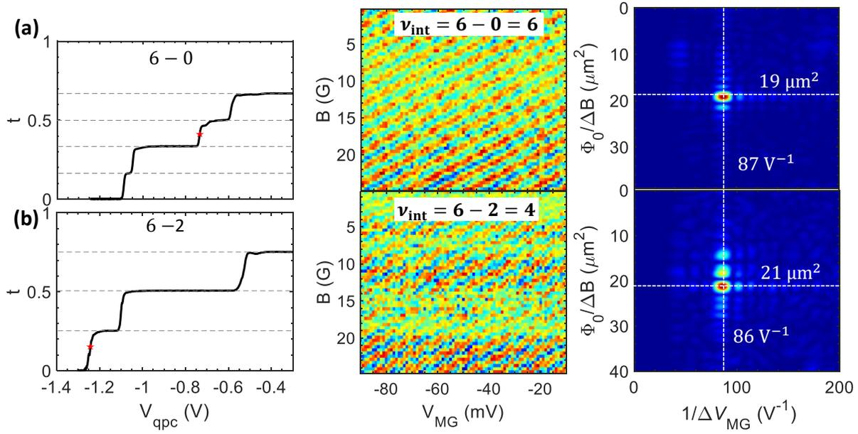
**Figure S7 | Results at bulk filling of  $\nu_b = 6$ .** The transmission in a QPC showing equispaced integer plateaus, and the interfering LL2 mode marked by the star symbol for (a)  $6 - 0 = 6$ , and (b)  $6 - 2 = 4$  interface configurations. The AB interference patterns and the FFTs are shown on the right. For both cases, the frequencies show pairing, irrespective of whether two LL1 modes are fully gapped out or fully transmitted through the FPI.
