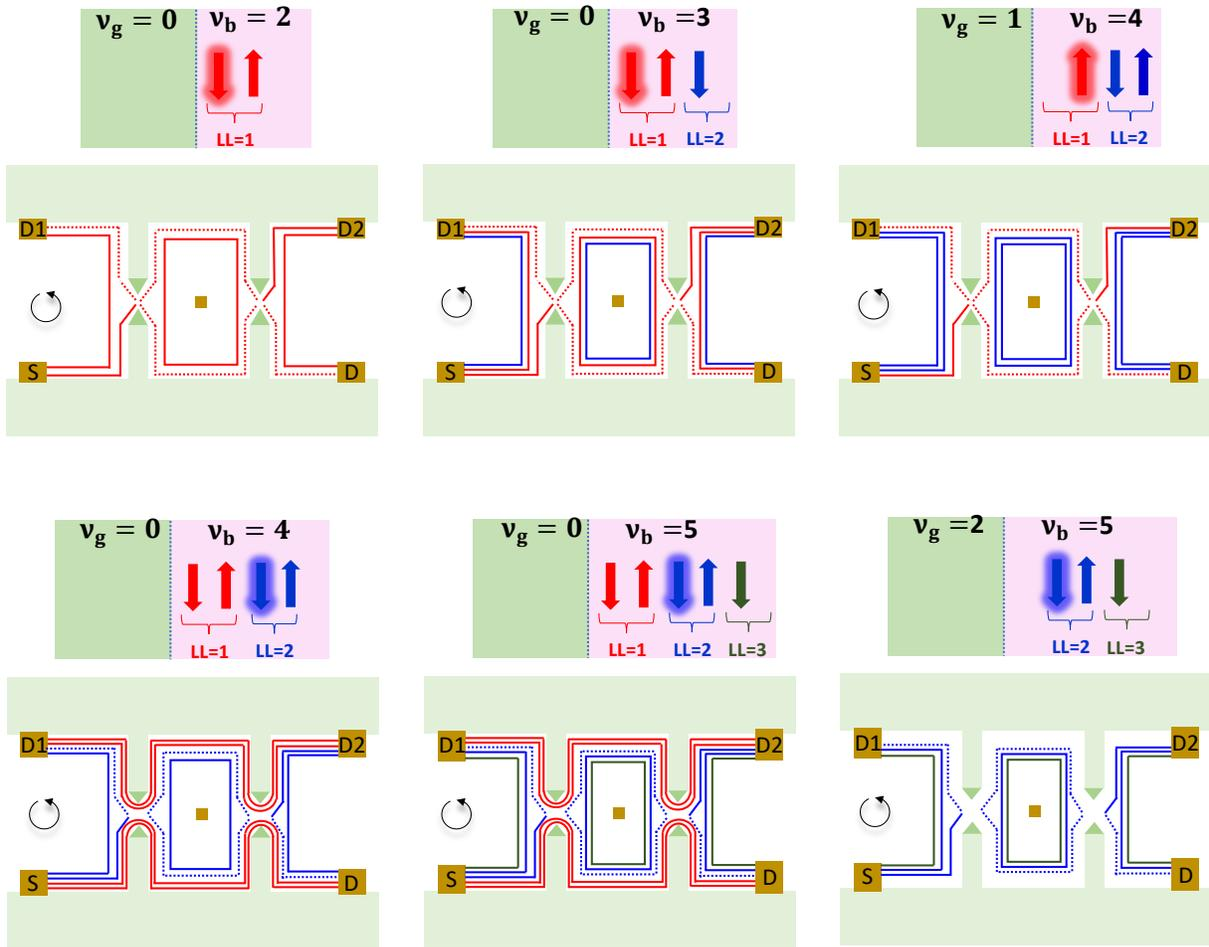
**Figure S3 | Edge-mode schematics for various interference configurations:** Schematics of the edge modes propagation around the gates, and inside the interferometer for different interference conditions. The respective LL (spin) modes with the interfering one glow are shown on top.
