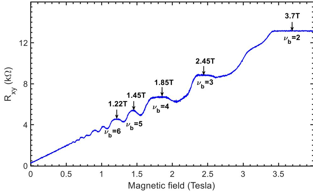
**Figure S2 | Hall measurement of the bulk.** Two terminal Hall resistance ( $R_{xy}$ ) of the bulk as a function of the magnetic field ( $B$ ) showing the QH plateaus. The bulk filling factors from  $\nu_b = 2$  to 6 are marked with the respective  $B$  value at which the measurements were performed.
