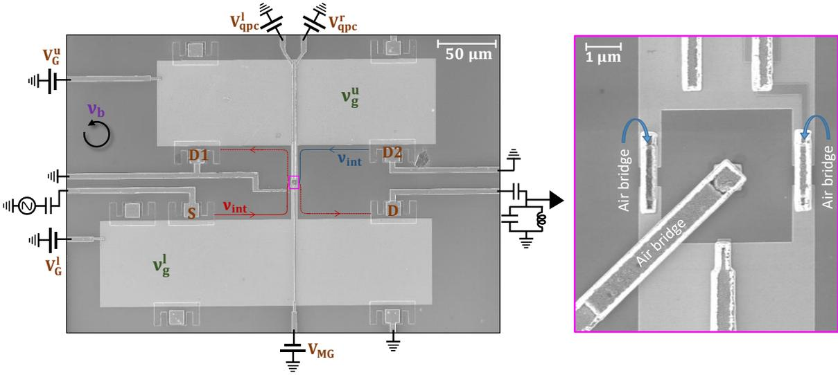
**Figure S1 | Large-scale SEM image of the device.** Left: SEM image of the whole device structure with various ohmic contacts, gates, and leads. Right: A zoomed image of the FPI showing the air bridge connections on the QPCs and the center ohmic contact. A partial broken lead from the left QPC is to be ignored.
