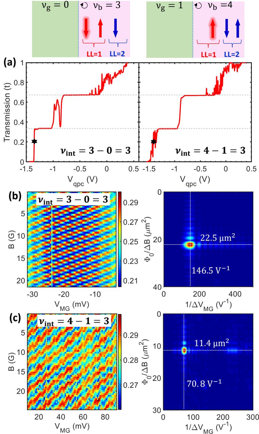
**Figure 3 | Outer edge interference for two types of engineered  $\nu_{\text{int}} = 3$ , namely,  $3 - 0 = 3$  and  $4 - 1 = 3$ .** (a) The transmission ( $t$ ) in a quantum point contact (QPC) as a function of the QPC-gate-voltage  $V_{\text{qpc}}$  showing three plateaus for both conditions for  $\nu_{\text{int}} = 3$ . The star symbol represents a typical partitioning of the outer mode for interference. The schematics on top represent
