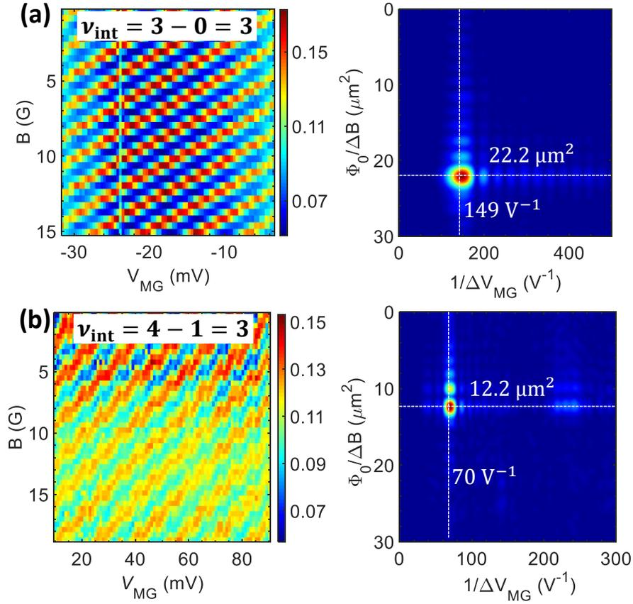
**Figure S4 | Outer edge interference for  $\nu_{\text{int}} = 3$ , when QPCs are relatively pinched.** The characteristic AB pyjamas and their FFT for (a)  $3 - 0 = 3$  with pairing, when  $t \approx 0.57$ , and (b)  $4 - 1 = 3$  without pairing, when  $t \approx 0.57$ .
