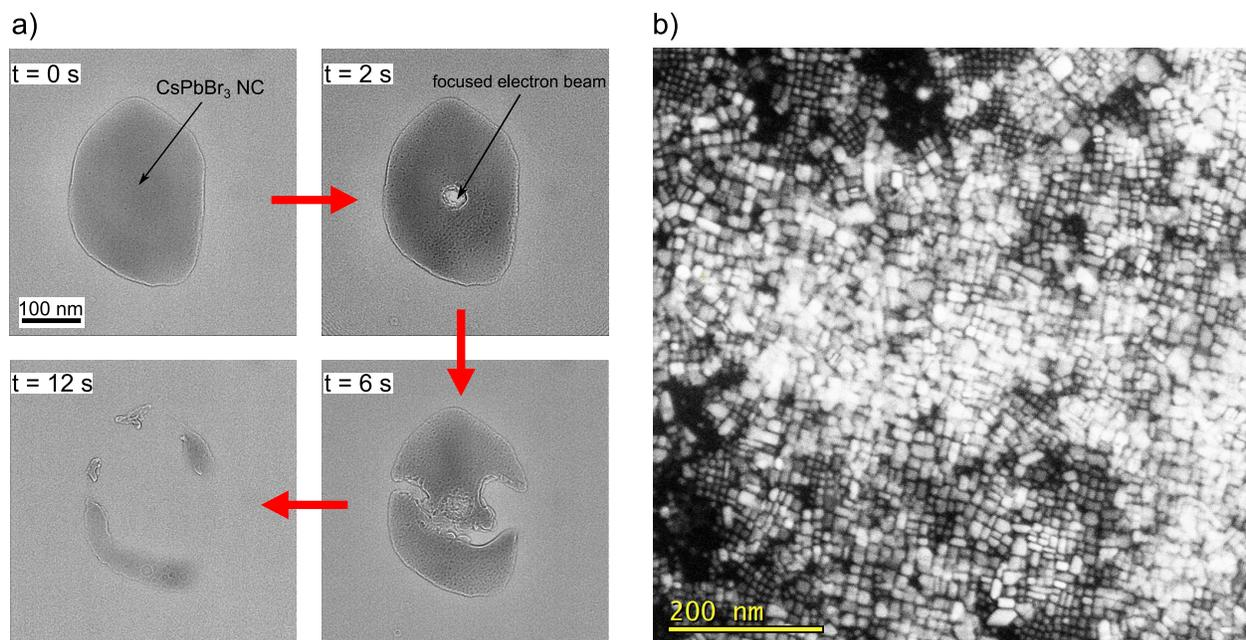
Figure S3: a) Immediate degradation of drop casted CsPbBr<sub>3</sub> NCs in TEM observation under focused electron beam. b) Overview STEM image of colloidal CsPbBr<sub>3</sub> NCs serving for the crystal lattice acquisition.
