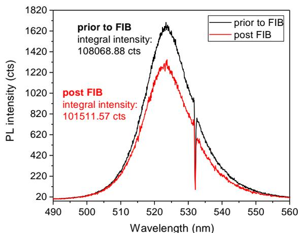
Figure S2: Prior to FIB processing and post FIB processing obtained typical PL integral intensities of CsPbBr<sub>3</sub> NC.
