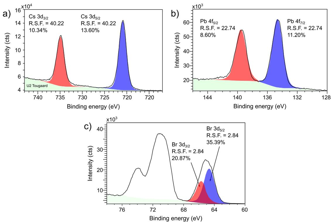
Figure S4: XPS spectra for determination of the stoichiometry of a) Cs, b) Pb, and c) Br atoms.
