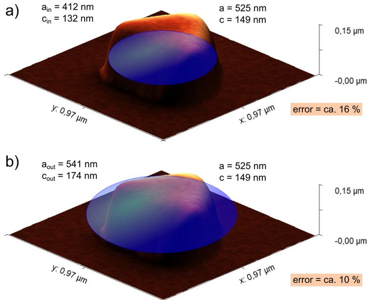
Figure S5: a) Inscribed and b) circumscribed spheroid compared to the effective length and height of the NC.
