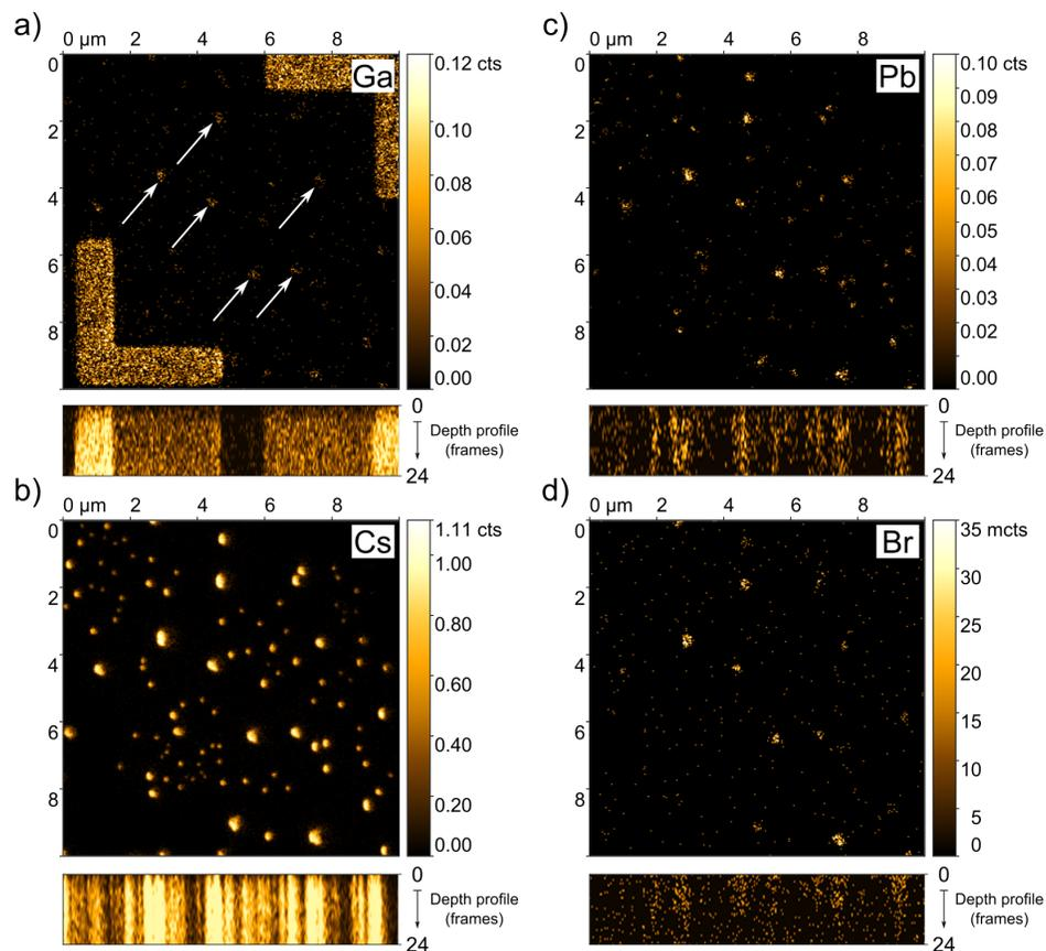
Figure 2: a) Analysed region on the sample used for the 3D elemental mapping of Ga, b) Cs, c) Pb and d) Br atoms. The white arrows in a) show the Ga ion implementation into the CsPbBr<sub>3</sub> NCs. The intensity of the signal obtained by ToF-SIMS in b)–d) does not indicate any inhomogeneity in the spatial or depth elemental distribution. This assumption is based on a comparison of ToF-SIMS signals between NCs with similar volumes.
