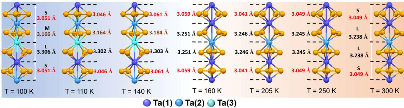
Figure A1. *Ta* metal bonding sequence in *n*-TSI: Metal bonding sequence, obtained from SXRD data, along each  $\text{TaSe}_4$  chain at  $T = 100$  K, 110 K, 140 K, 160 K, 205 K, 250 K, and 300 K.
