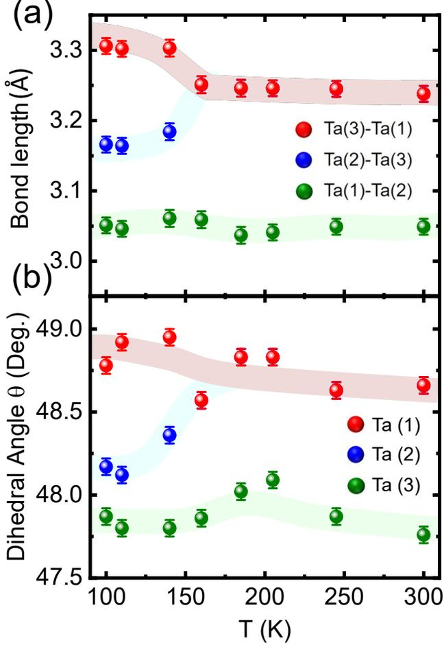
Figure 3. (a) Temperature variation of Bond distance among different Ta atoms and (b) dihedral angle. The solid sphere represents the experimental data, while thick solid lines are the guide to the eye.
