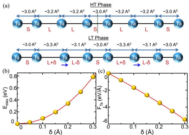
Figure 5. (a) The schematic diagram of the distribution of Ta-Ta bond lengths in the  $\text{TaSe}_4$  chain in HT and LT crystal structure. The center of inversion (marked as a dotted line) in the HT structure, gets broken in the LT structure due to the distortion  $\delta$ . Elastic energy (b) and force acting on Ta ions (c) plotted as a function of off-centric displacement ( $\delta$ ), obtained from DFT calculations.
